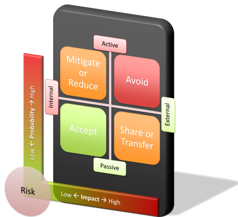
Fig. 10. Risk, risk response choices (accept, share or transfer, avoid, mitigate or reduce) and their types (active vs. passive) and scopes (internal vs. external)
