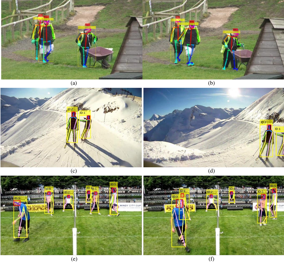
Şekil 8. Örnek birer videoda OpenPose ile videonun (a) 22. ve (b) 40. karelerinde, DCPose ile videonun (c) 53. ve (d) 77. karelerinde, DCPose ile videonun (e) 84. ve (f) 149. karelerinde bulunan kişilerin takip sonuçları (In an example videos video tracking results of the OpenPose at (a) 22 nd and (b) 40 th frames of the video, DCPose at (c) 53 rd and (d) 77 th frames of the video, and DCPose at (e) 84 th and (f) 149 th frames of the video)
