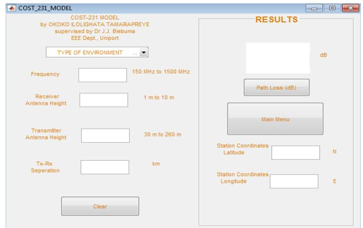
**Fig. 3.** The Developed Model Interface of COST-231 Hata for path loss analysis.
