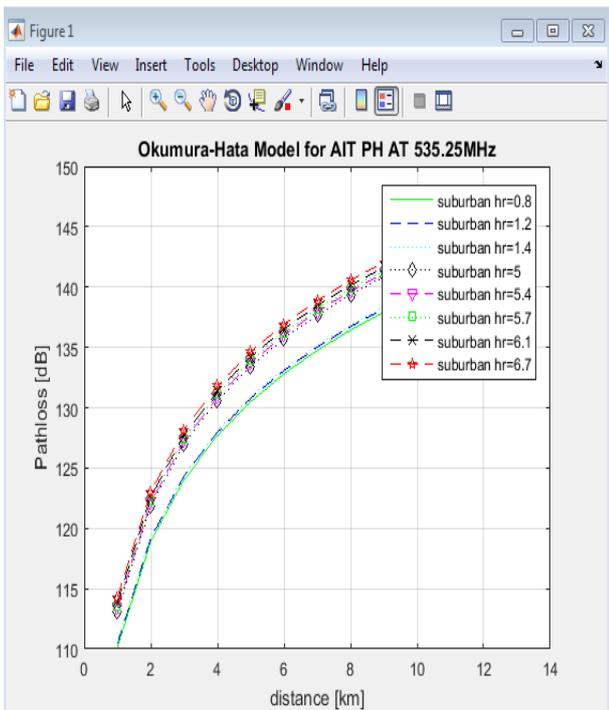
**Fig 4.** Path loss vs distance for AIT PH @ 535.25MHz using Okumura-Hata Model
