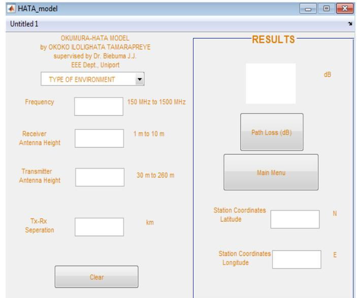
**Fig. 2.** the Developed Model Interface of Okumura-Hata for path loss analysis
