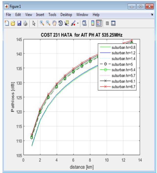
**Fig 5.** Path loss vs distance for AIT PH @ 535.25 MHz using COST-231 Hata Model
