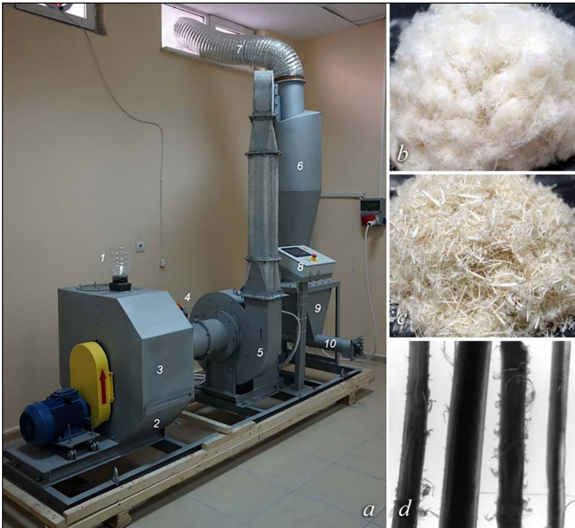
Figure 3. a) machine for separating the feather into the fiber and the rachis; b) separated feather fiber; c) separated feather rachis pieces; d) view of the pieces of rachis under the microscope after cutting the fibrous part of the feather
