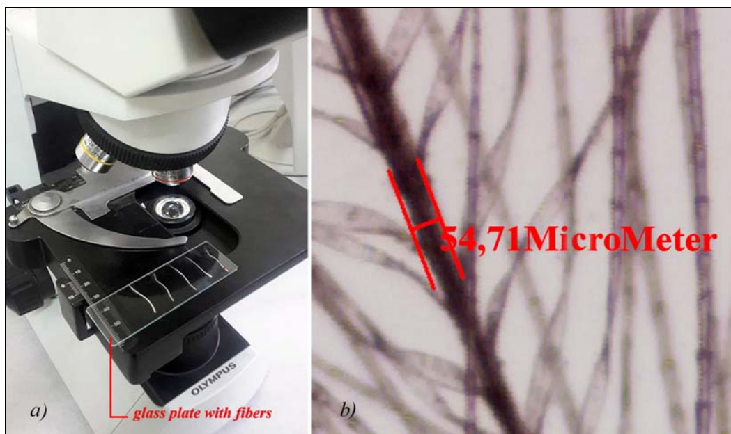
Figure 4. Measuring fiber length and thickness with a microscope: a) microscope and glass plate with fiber, b) fiber under the microscope
