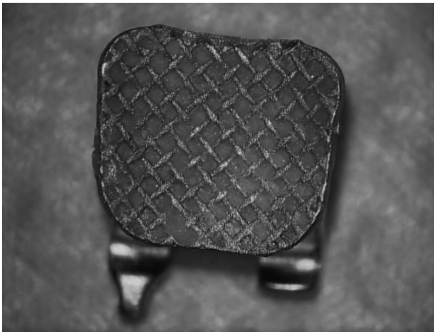
Figure 2. The base of each bracket was examined by stereomicroscope (Lumera T, Carl Zeiss AG, Oberkochen, Germany) at 20x magnification and an ARI score was determined according to the criteria defined by Artun and Bergland. 19
