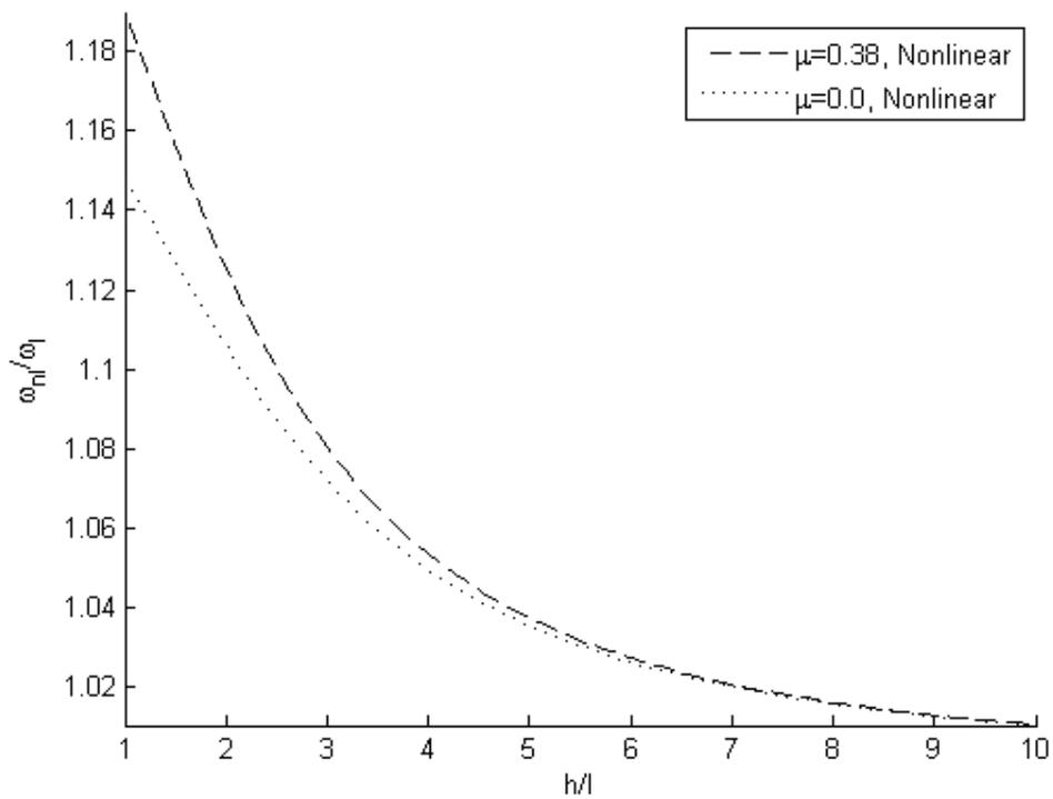
Fig. 2. The ratio of the non-classical frequency to the linear classical frequency as a function of  $h/l$ .
