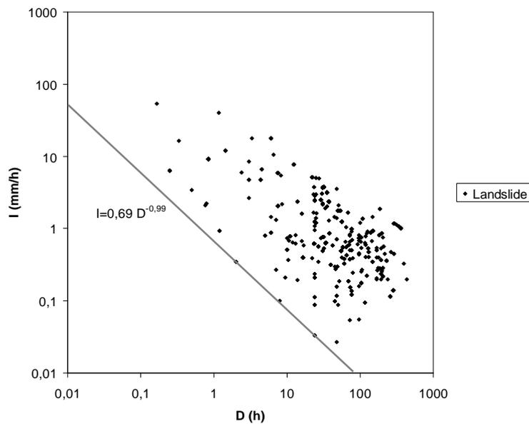
Fig. 4. Rainfall threshold triggering landslides in Trabzon province
