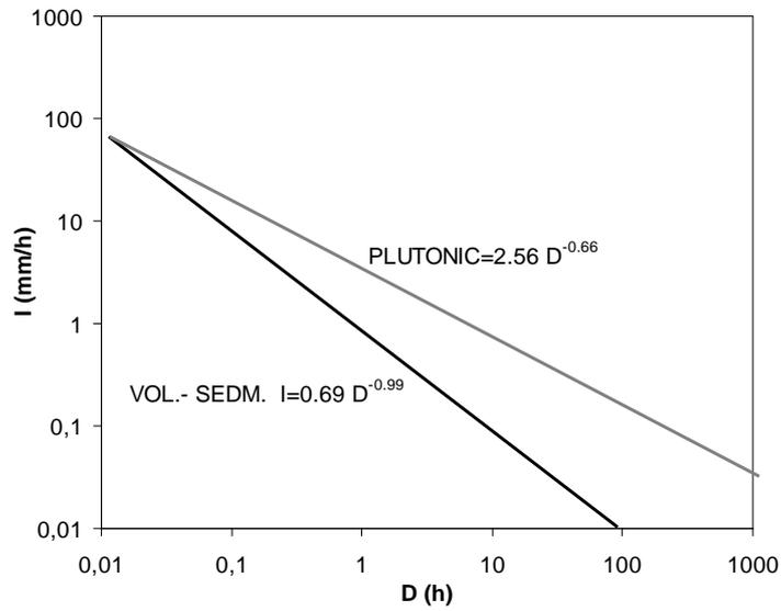
Fig. 8. Landslide-rainfall intensity- according to rock type
