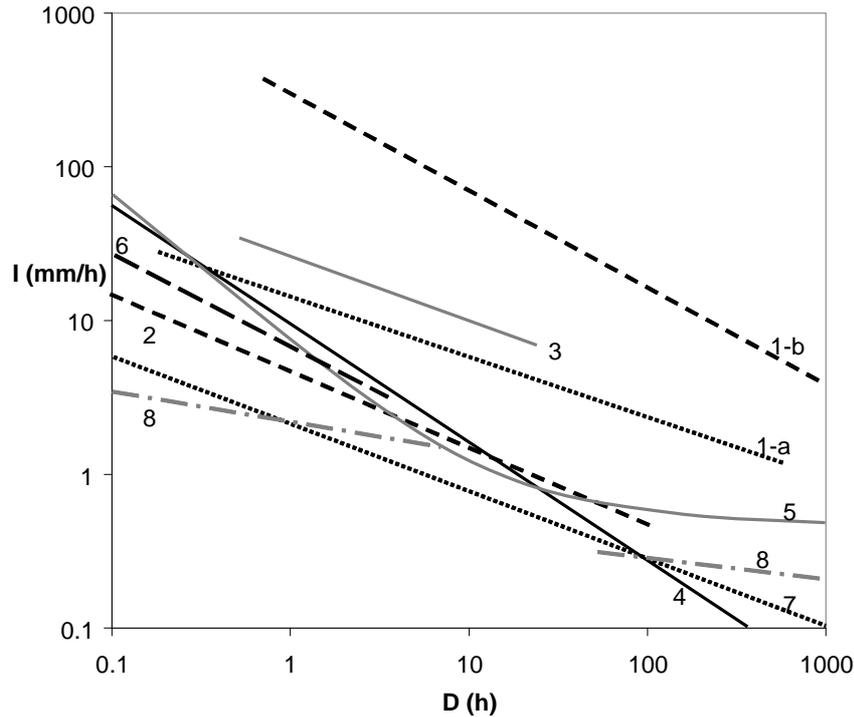
Fig.1. Comparison of the global intensity-duration (ID) thresholds. 1-a. Minimum rainfall threshold Caine [9]; 1-b. Maximum rainfall threshold Caine [9]; 2. Innes [10]; 3. Jibson RW [11] 4. Clarizio, Gulli & Sorbino [12]; 5. Crosta & Frattini [5]; 6. Cannon & Gartner [13]; 7. Guzzetti & Peruccacci [14]; 8. Thresholds obtained for two different rainfall periods Guzzetti & Peruccacci [14]
