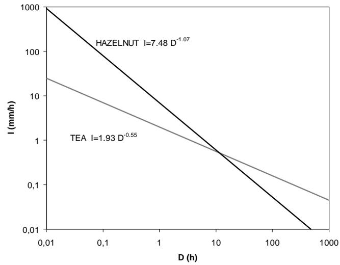
Fig. 10. Landslide-rainfall intensity-duration according to type of agricultural product
