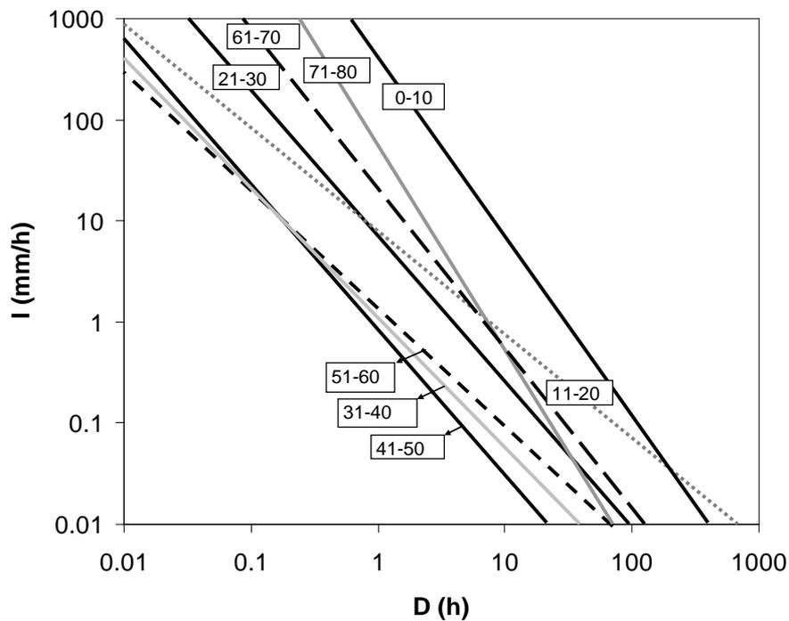
Fig. 6. Landslide- rainfall intensity-duration according to slope angles
