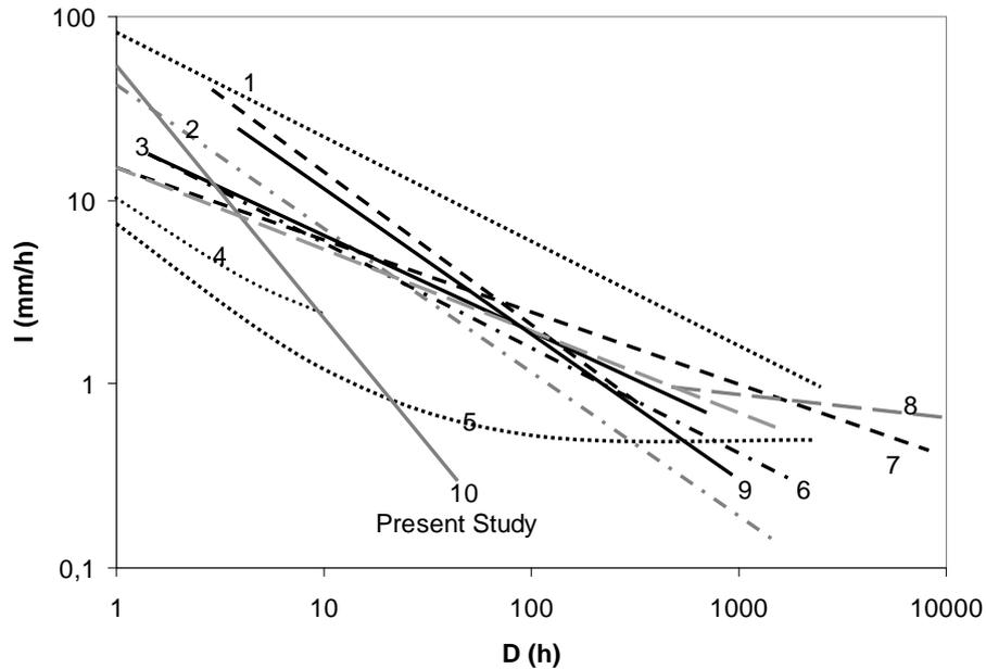
Fig. 11. Comparison of landslide–rainfall thresholds (Numbers refer to # in table 3)
