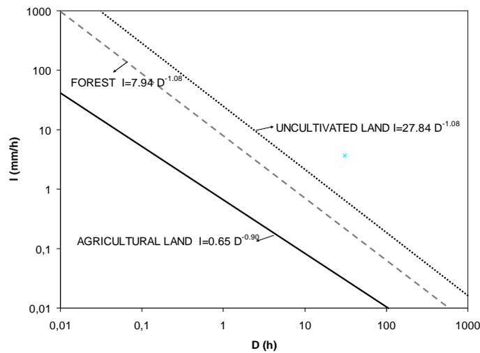
Fig. 9. Landslide-rainfall intensity-duration according to cover type
