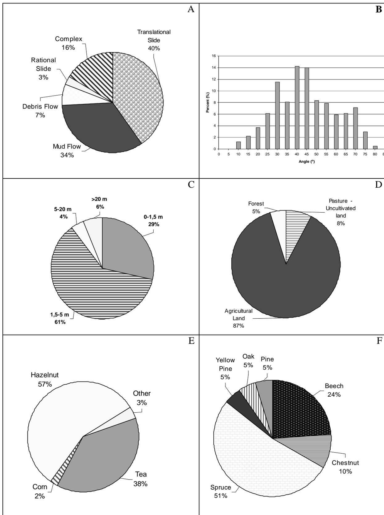
Fig. 3. Categorization of the landslides in Trabzon province (A) landslide type (B) natural slope angles (C) thickness of sliding mass (D) cover type (E) type of agricultural product (F) type of tree
