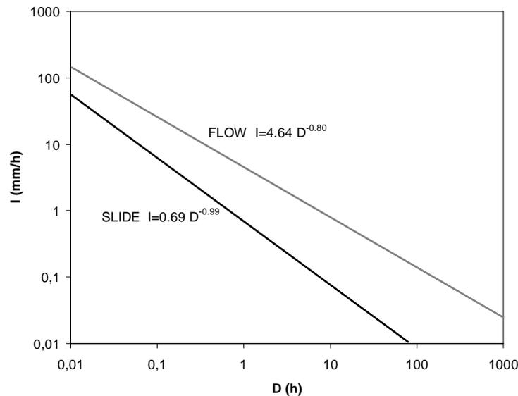
Fig. 7. Landslide-rainfall intensity-duration according to landslide type
