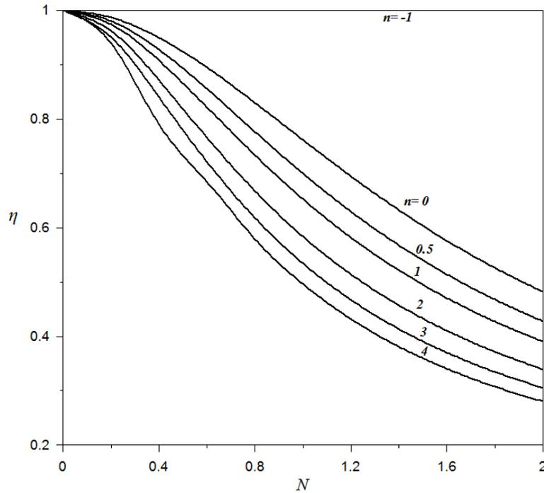
Fig. 4. variation of fin efficiency with  $N$  for several assigned values of  $n$
