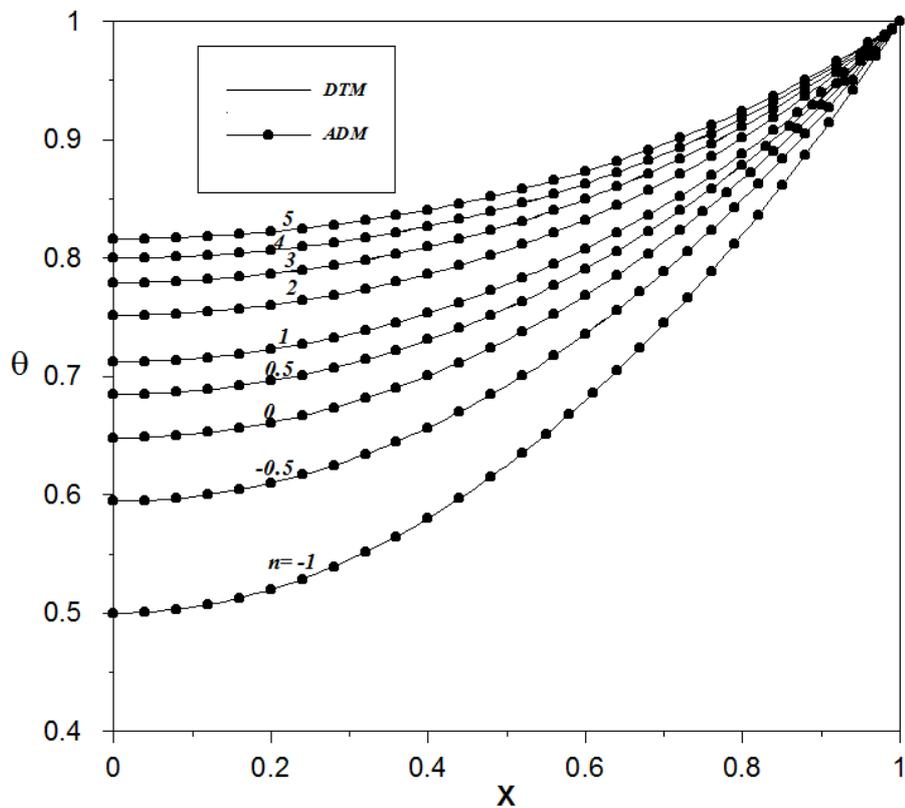
Fig. 2. Temperature profile for several assigned value of  $n$  at  $N=1$
