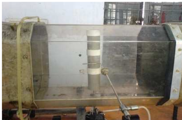
Fig. 2. Photograph of wind tunnel test section
