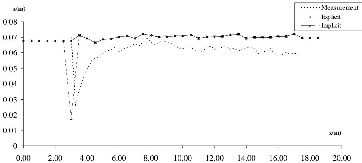
**Fig. 9.** Comparison of experimental and numerical results for bed profile in Hydrograph 1
