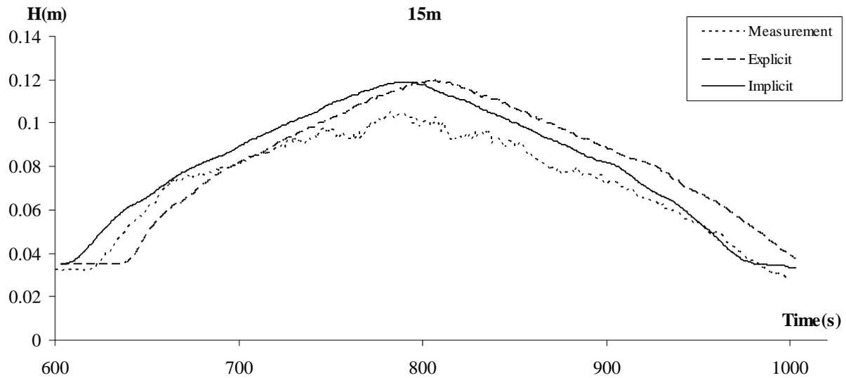
**Fig. 10d.** Comparison of flow depth for hydrograph 2 in  $x=15\text{m}$
