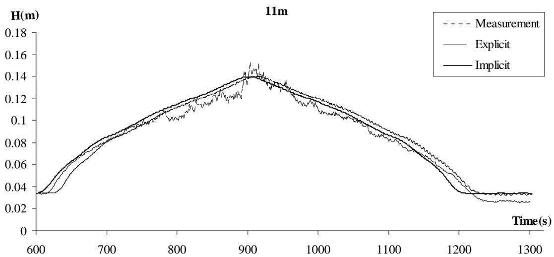
**Fig. 8c.** Experimental and numerical results for flow depth in  $x=11\text{m}$  and Hydrograph 1
