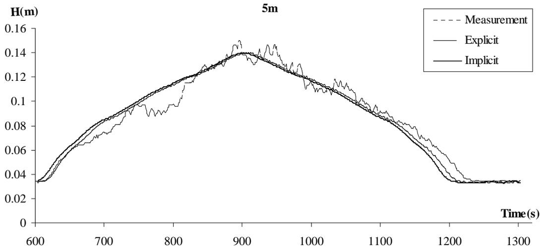
**Fig. 8a.** Experimental and numerical results for flow depth in  $x=5\text{m}$  and Hydrograph 1
