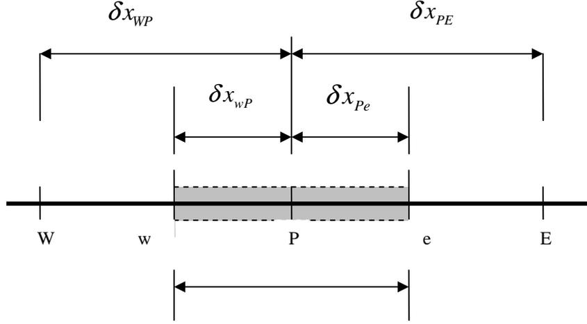
**Fig. 2.** Illustration of finite volume method in one dimensional
