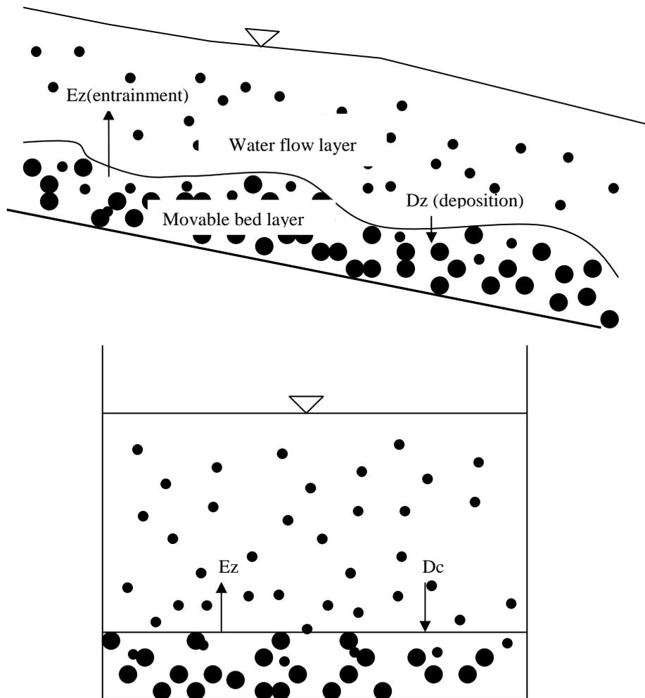
**Fig 1.** Schematic representation of two layer system
