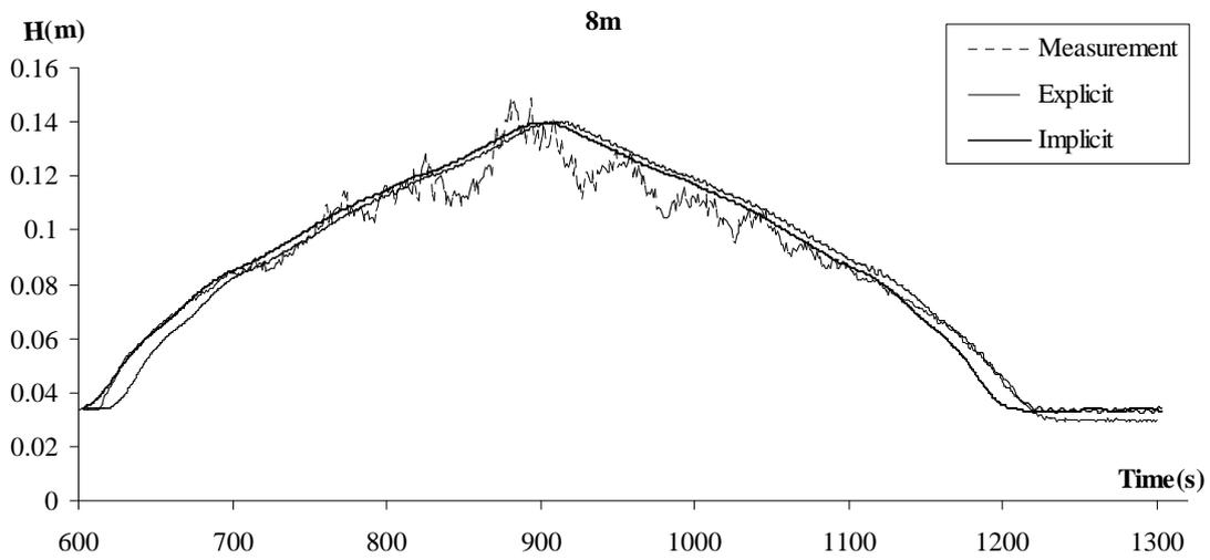
**Fig. 8b.** Experimental and numerical results for flow depth in  $x=8\text{m}$  and Hydrograph 1
