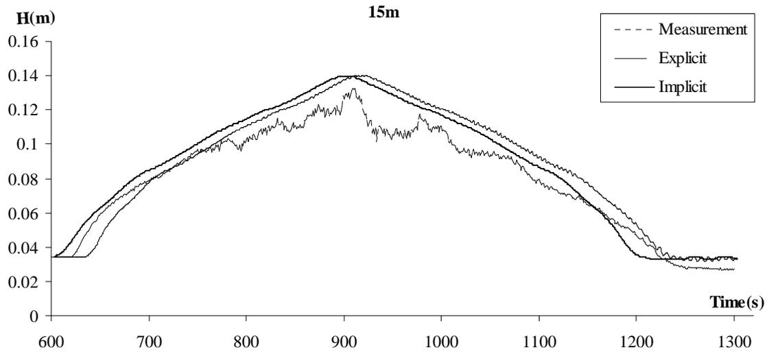
**Fig. 8d.** Experimental and numerical results for flow depth in  $x=15\text{m}$  and Hydrograph 1
