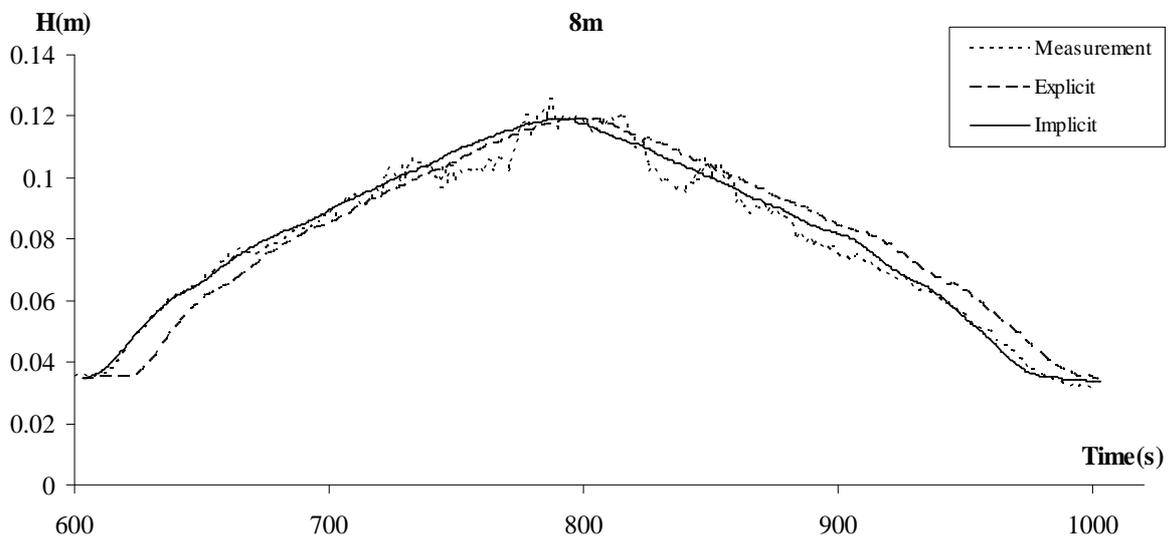
**Fig. 10b.** Comparison of flow depth for hydrograph 2 in  $x=8m$
