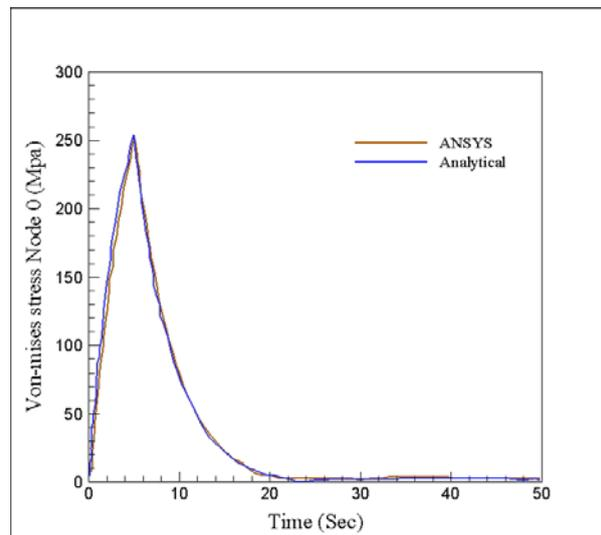
Figure 3. Comparison of effect of thermal and pressure loading on Von-mises at 8 nodes stress for two methods
