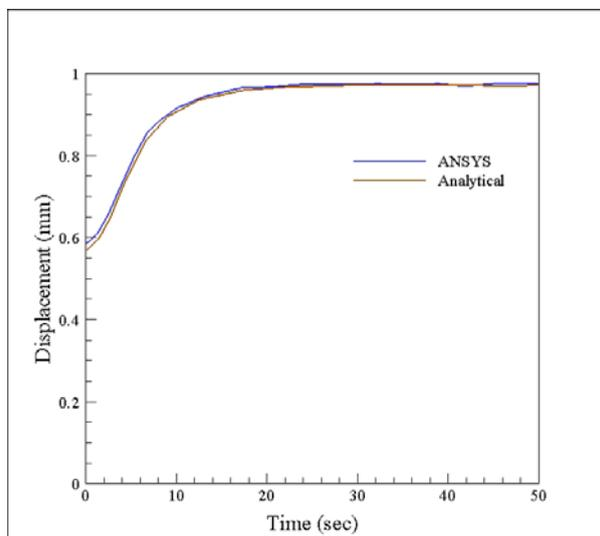
Figure 4. Comparison of effect of thermal and pressure loading on displacement for two methods
