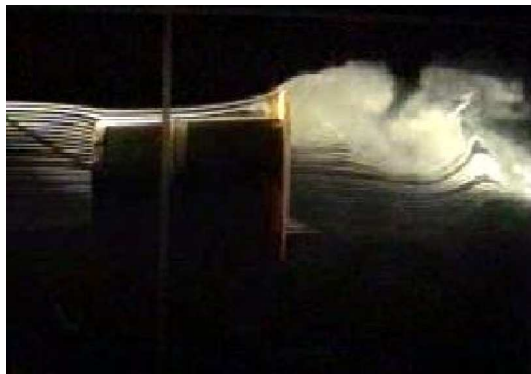
Figure 4. Flow around a circular-diffuser model with a brim. The smoke flows from left to right. L/D = 1.5 . The area ratio \mu (outlet area/inlet area) of the circular-diffuser model is 1.44. Karman vortices are formed behind brim.
