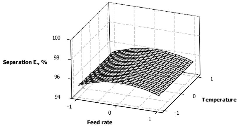
Fig.9(c). Response surface plots showing the effect of feed rate ( $f$ ) and temperature ( $t$ ) on the separation efficiency
