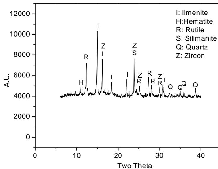
Fig.3. XRD of deslimed feed sample
