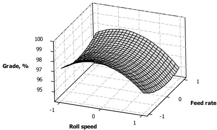
Fig.7(a). Response surface plots showing the effect of roll speed ( $v$ ) and feed rate ( $f$ ) on the grade
