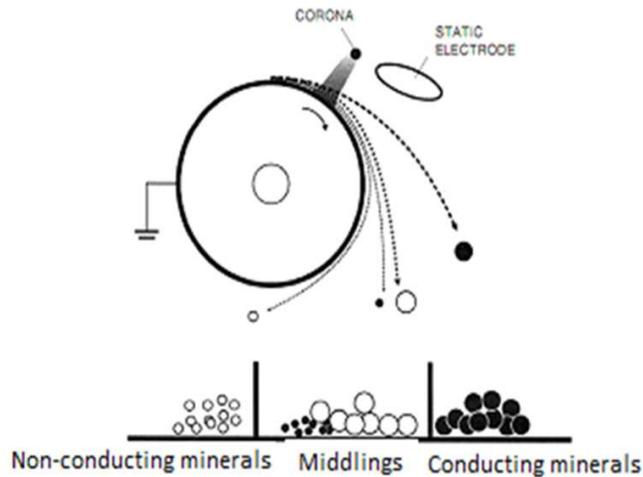
Fig.1. Principles of operations for High Tension Roll Separator to recover conducting minerals
