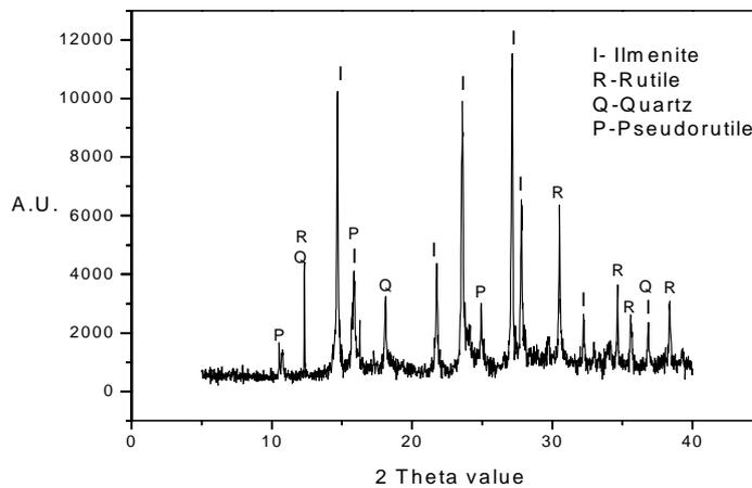
Fig.10. XRD pattern of conducting fraction achieved from HTRS
