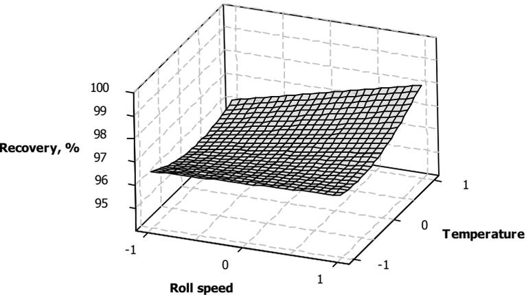
Fig. 8(b). Response surface plots showing the effect of roll speed ( $v$ ) and temperature ( $t$ ) on the recovery
