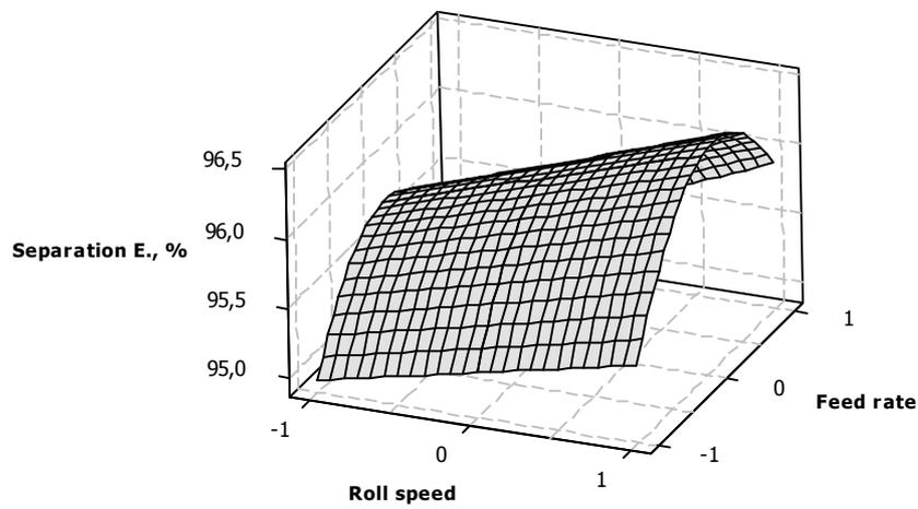
Fig.9(a). Response surface plots showing the effect of roll speed ( $v$ ) and feed rate ( $f$ ) on the separation efficiency
