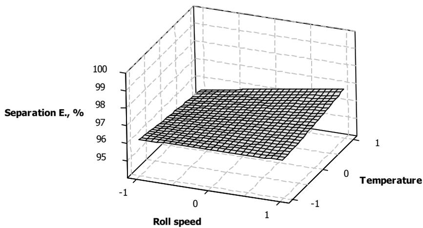
Fig. 9(b). Response surface plots showing the effect of roll speed ( $v$ ) and temperature ( $t$ ) on the separation efficiency
