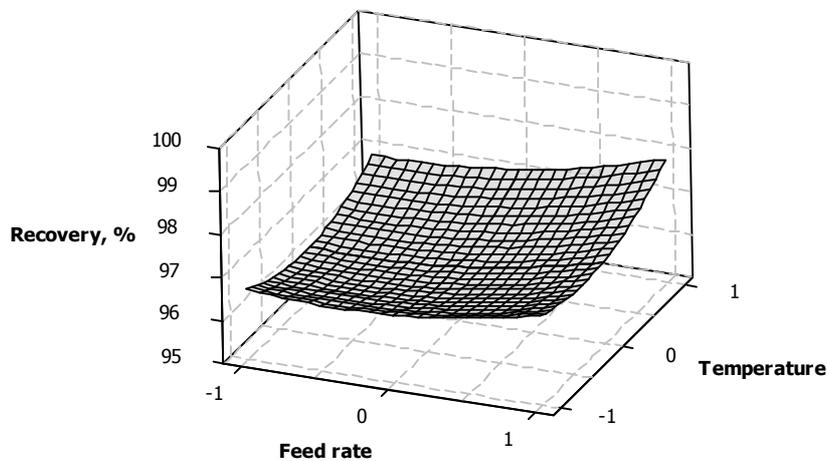
Fig.8(c). Response surface plots showing the effect of feed rate ( $f$ ) and temperature ( $t$ ) on the recovery
