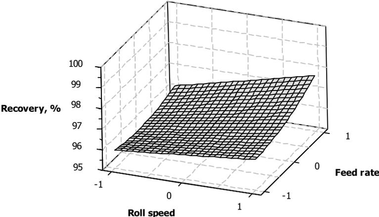
Fig.8(a). Response surface plots showing the effect of roll speed ( $v$ ) and feed rate ( $f$ ) on the recovery
