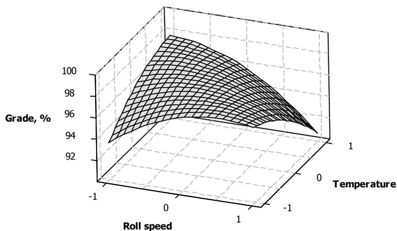
Fig. 7(b). Response surface plots showing the effect of roll speed ( $v$ ) and temperature ( $t$ ) on the grade
