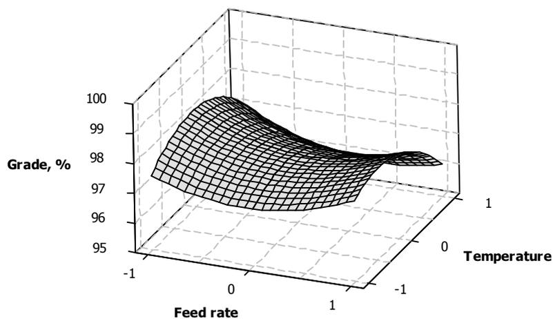
Fig. 7(c). Response surface plots showing the effect of feed rate ( $f$ ) and temperature ( $t$ ) on the grade
