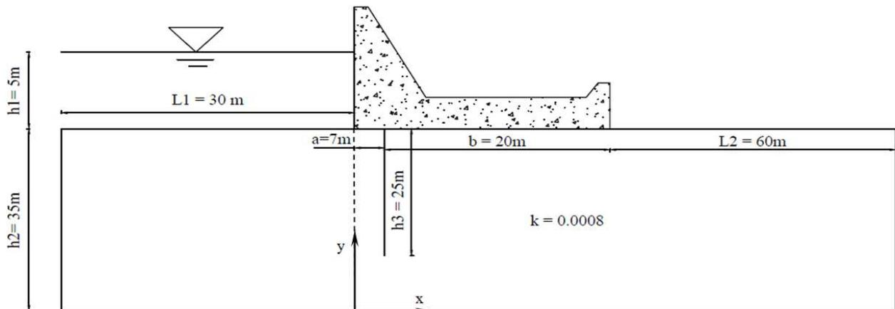
Figure 3. Characteristics of considered diversion dam
