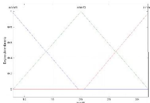
**Figure 12:** Typical Triangular Membership Function
