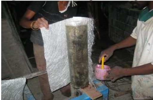
**Figure 2: Wrapping under Progress**
