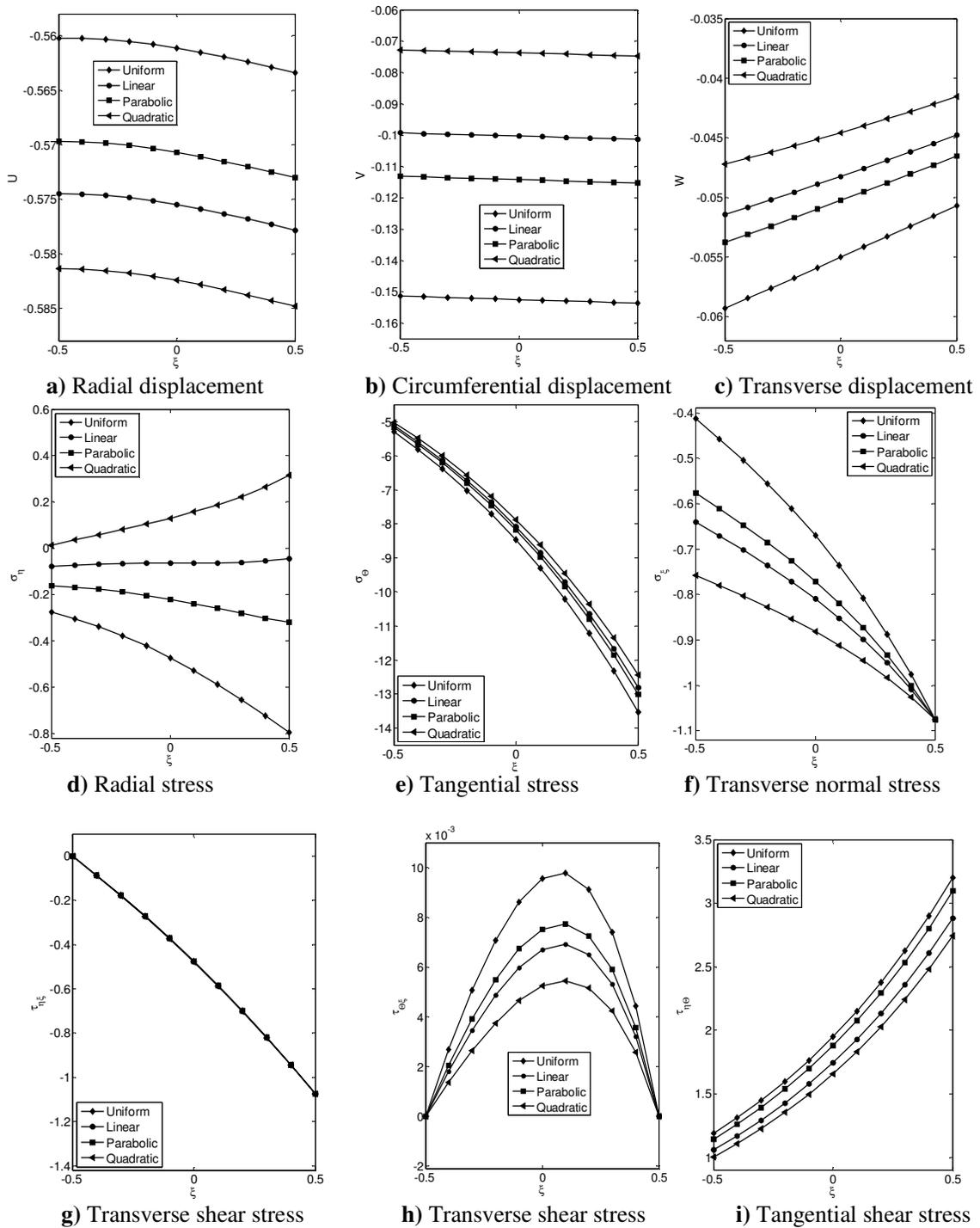
**Fig.8** Effect of various foundation patterns on variation of mechanical entities across the thickness direction for a clamped circular plate
