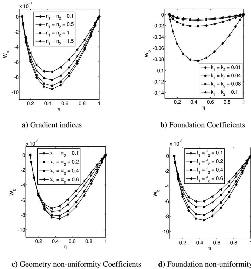
**Fig.9** Effect of various parameters on plate deflection at a location ( $\theta = 45^\circ$ )
