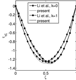
**Fig.2** Distribution of dimensionless transverse shear stress across the plate thickness at  $\eta = 0.5$
