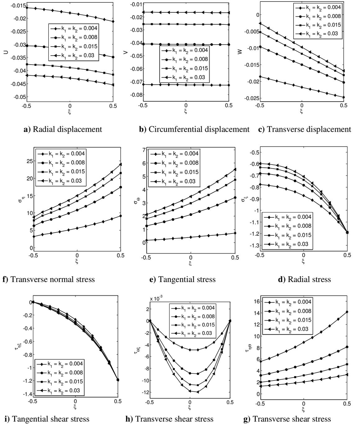
**Fig.6** Effect of the foundation coefficients on variation of mechanical entities across the plate thickness
