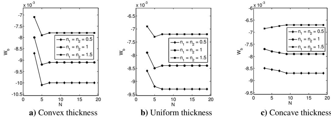
**Fig.3** Convergence of non-dimensional deflection of the plate at a location ( $\eta = 0.55, \theta = 45^\circ$ )
