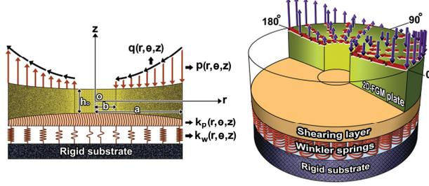
**Fig. 1** Geometry of non-uniform 2D-FGMs annular plate resting on gradient elastic foundations
