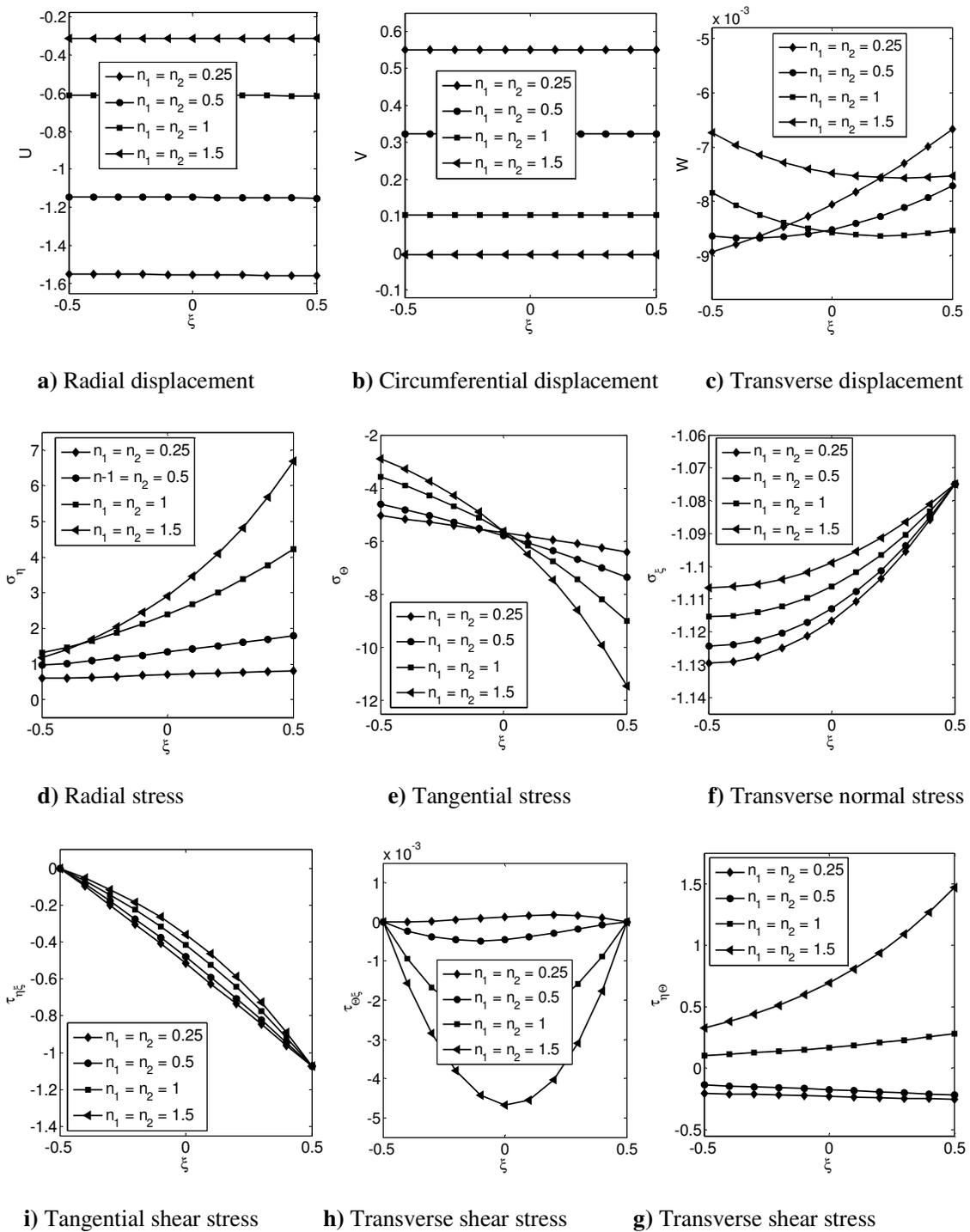
**Fig.4** Effect of the material heterogeneity indices on physical quantities across the plate thickness
