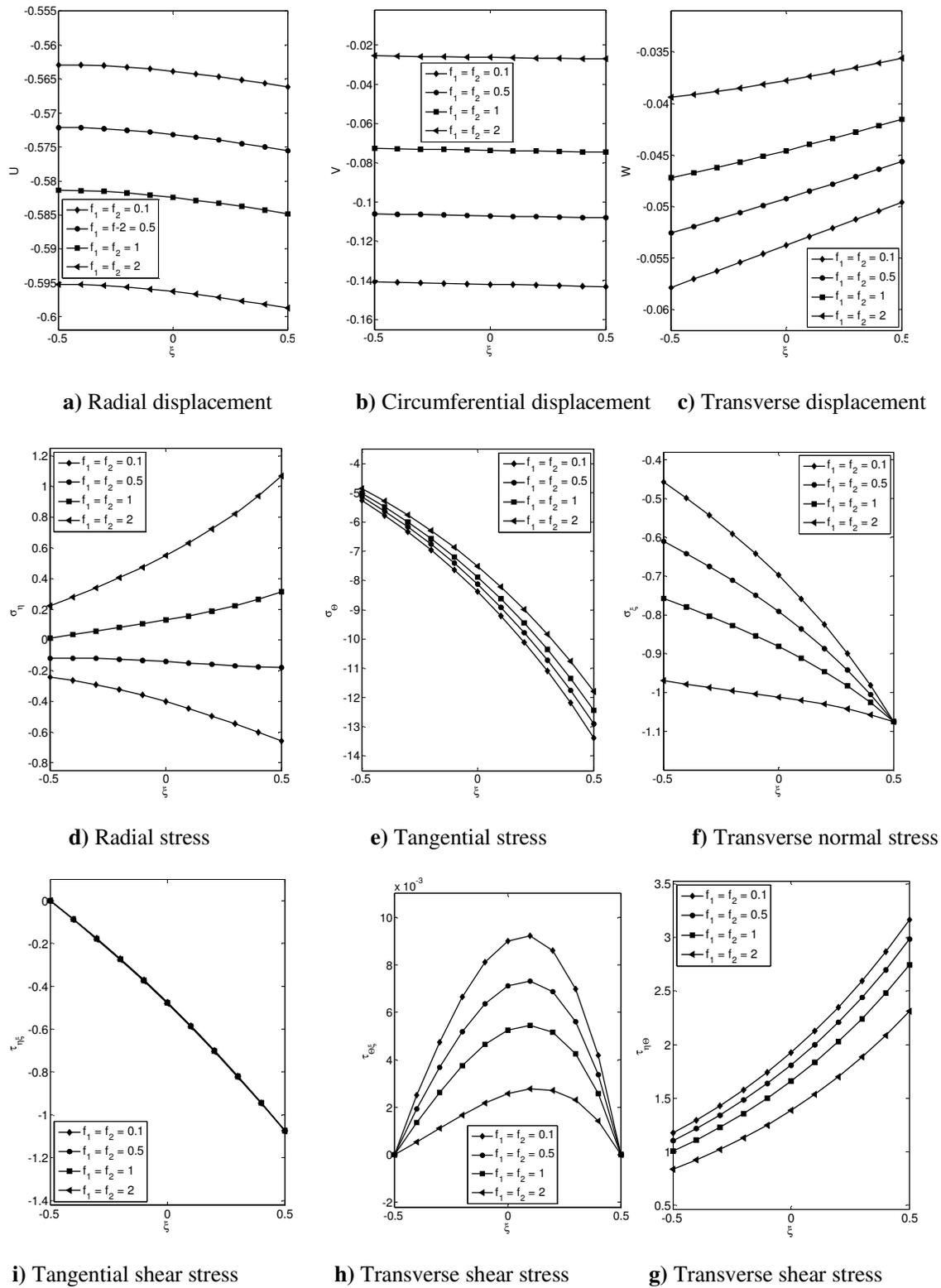
**Fig.7** Effect of foundation gradient indices on variation of mechanical entities across the plate thickness for a clamped circular plate
