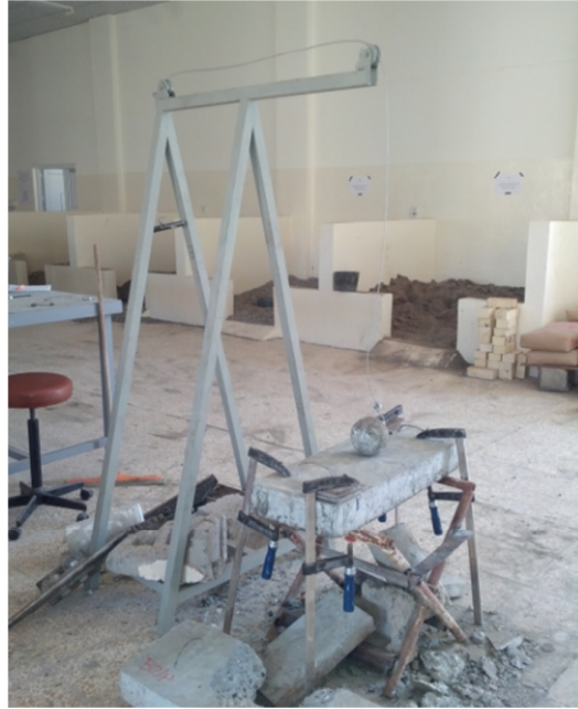
Figure 2: Present impact test for wide beam
