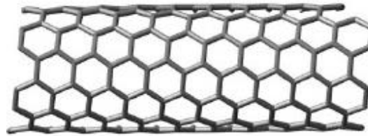
Fig. 1. Typical single-walled carbon nanotubes
