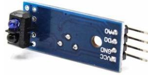
**Figure 4.** TCRT 5000 IR sensor card
