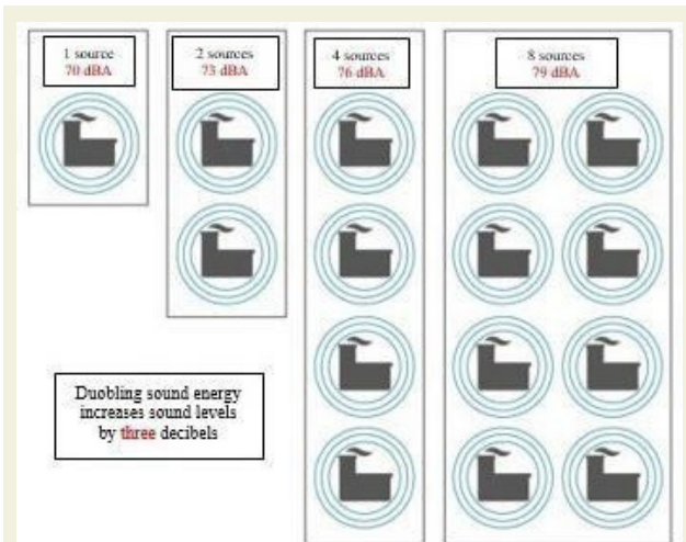
Figure 8. Change in sound pressure level when the number of sound sources is halved [86]
