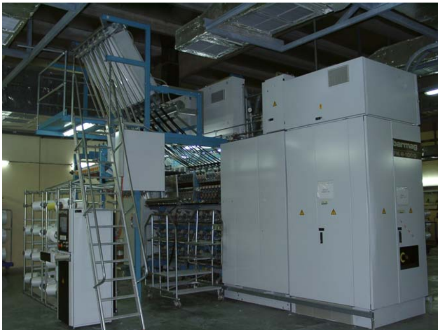
Figure 4. Barmag FK6 1000 pilot texturing machine
