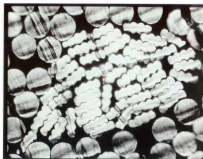
Figure 3. Six channels, 47 filaments, 133 decitex POY cross section
