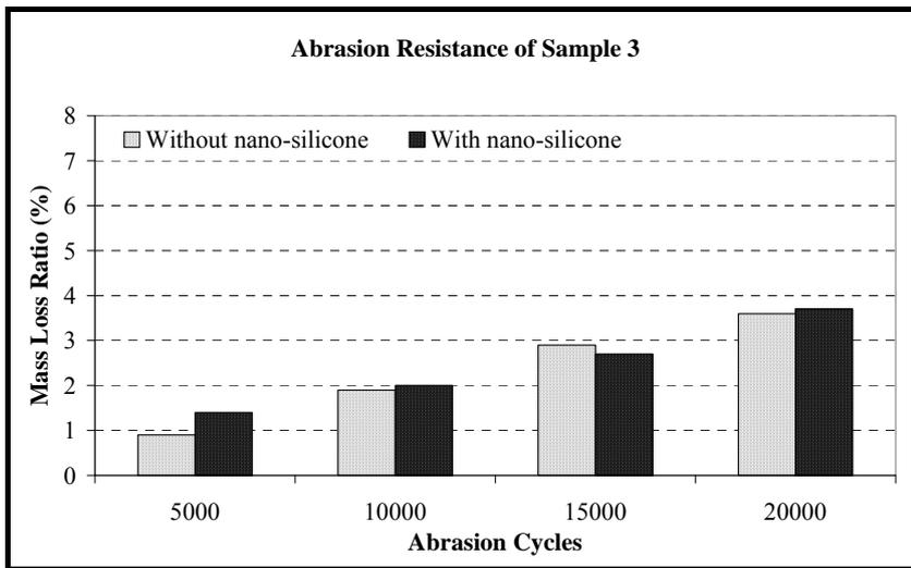
Figure 6. Abrasion resistance of sample 3
