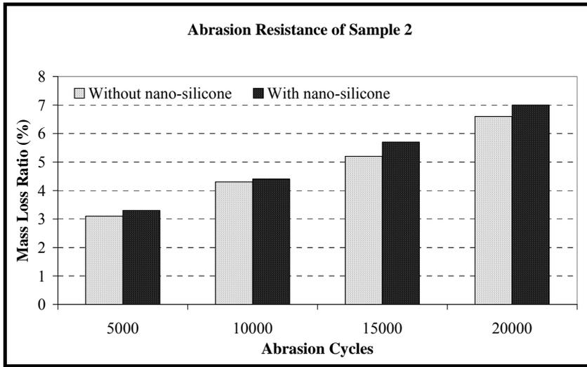
Figure 5. Abrasion resistance of sample 2
