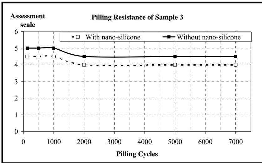
Figure 2. Pilling resistance of sample 3
