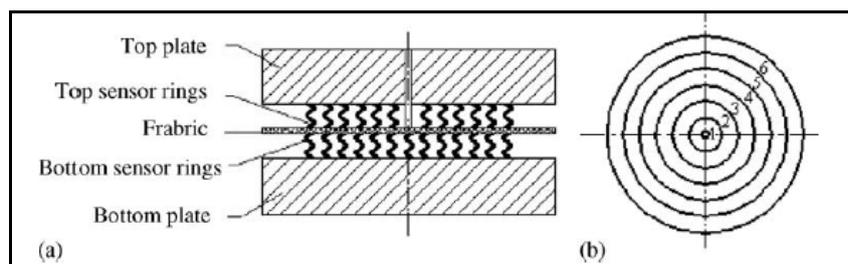
Figure 2. Sketch of MMT sensors: (a) sensor structure; (b) measuring rings (15).
