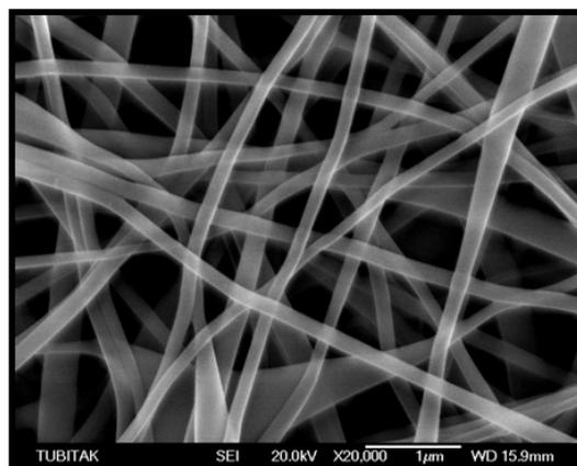
Figure 5. SEM image of the cross-linked nanofibrous mat immersed in water for 24 h. [X20.000]
