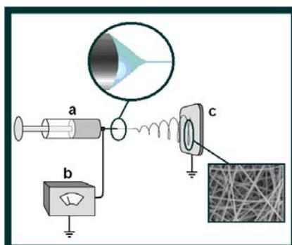
**Figure 1.** Schematic diagram of the electrospinning process (27)
