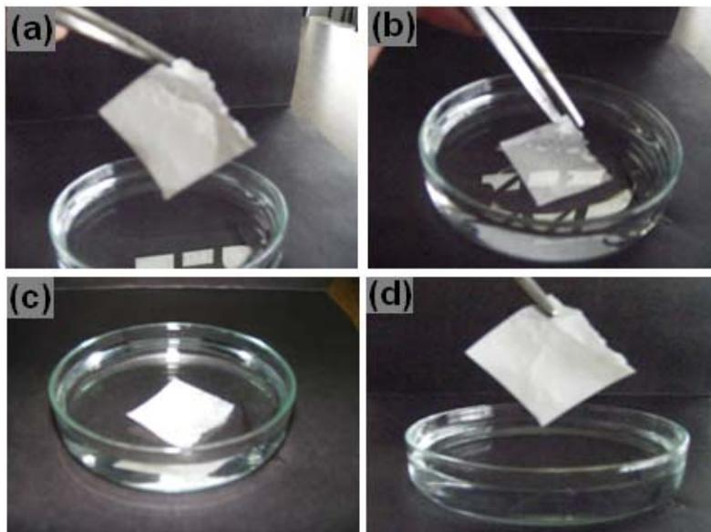
Figure 4. Water resistance test of the cross-linked nanofibrous mat [(a) Initial, (b) 1st s., (c) 3rd h. (d) After 24 h.]
