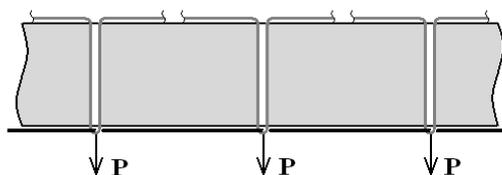
Figure 3. Extracting of the micro-wire from the stitch structure
