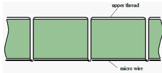
Figure 1. Insertion of the ferromagnetic micro-wire in the unbalanced lock-stitch structure
