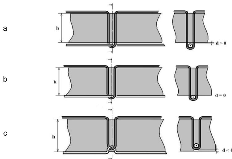
Figure 4. The aspect of the 301 lockstitch for different tensions of the upper thread
