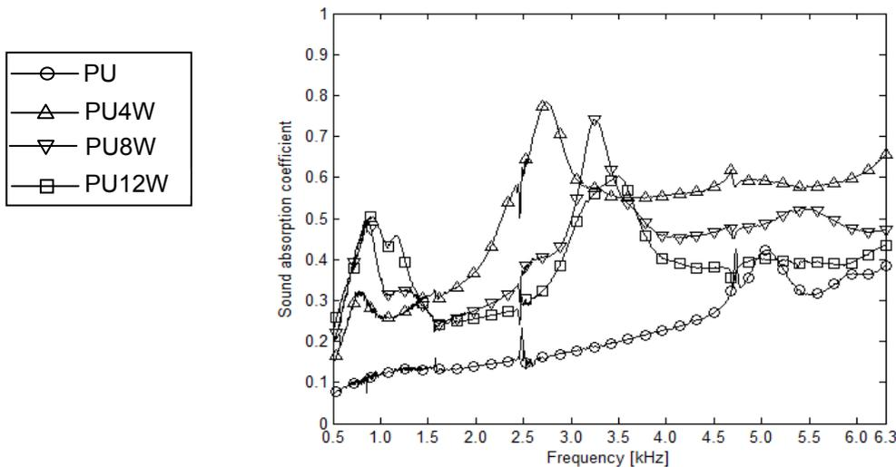
Figure 4. Sound absorption of PU foam and wool fiber composites
