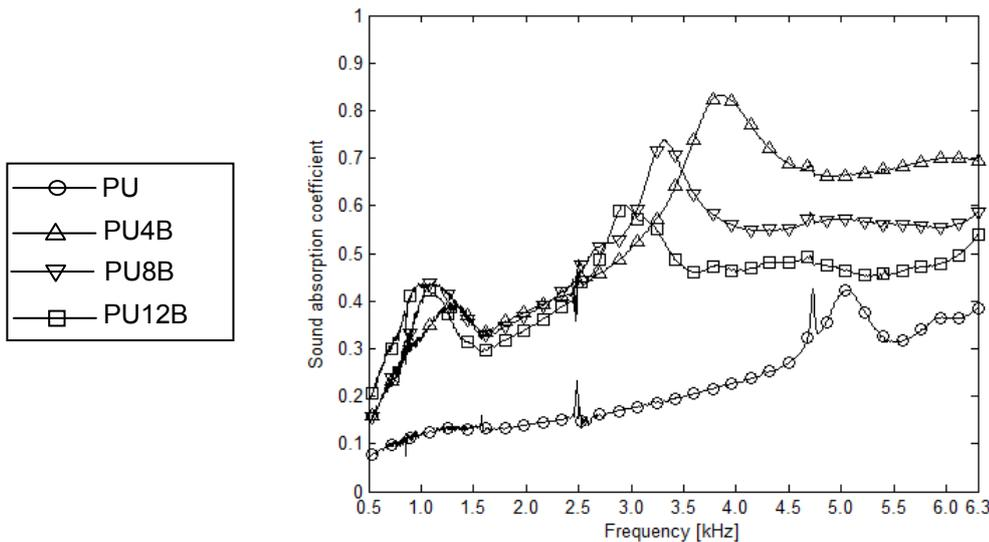
Figure 3. Sound absorption of PU foam and bamboo fiber composites
