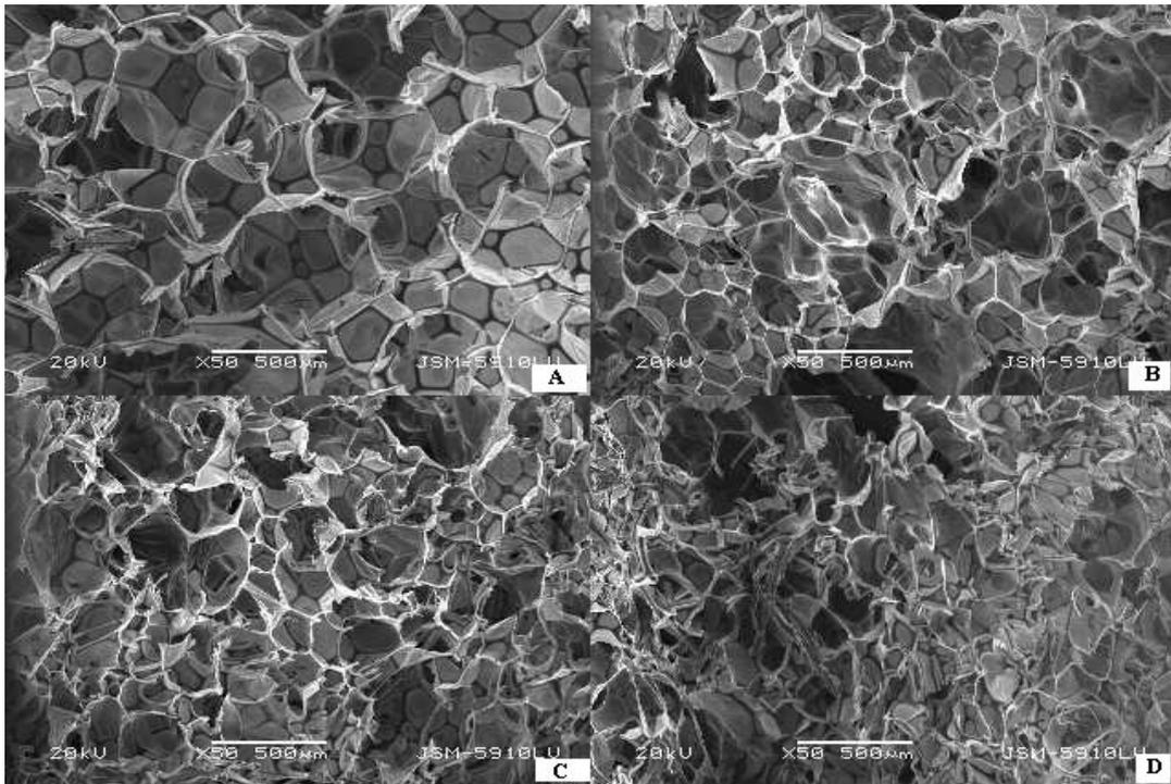
**Figure 9.** Cross-sectional SEM images of the PU foam with wool fiber additives (PUW). Magnification 50 x. A- standard PU foam, B- PU4W, C- PU8W, D- PU12W.
