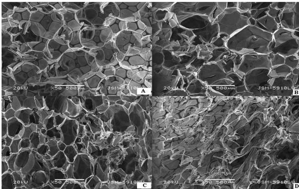
Figure 5. Cross-sectional SEM images of PU foam with cotton fiber additives (PUC). Magnification 50 x. A- standard PU foam, B- PU4C, C- PU8C, D- PU12C.
