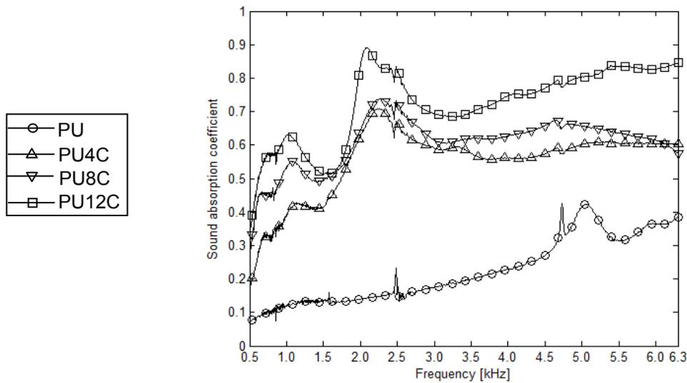
Figure 2. Sound absorption of PU foam and cotton fiber composites
