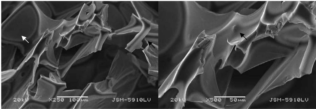
**Figure 8.** Cross-sectional SEM images of PU foam with bamboo fiber additives (PUB). Magnification 250 and 500 x.
