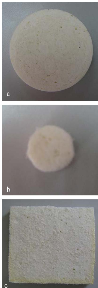
**Figure 1.** Samples prepared for acoustic and thermal measurements. (a) Sample for large tube sound absorption measurement, (b) sample for small tube sound absorption measurement.
