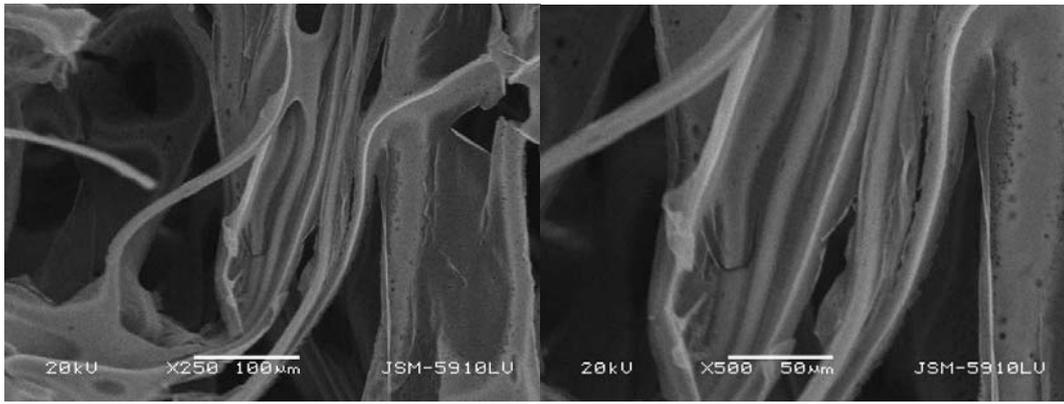
**Figure 6.** Cross-sectional SEM images of PU foam with cotton fiber additives (PUC). Magnification 250 and 500 x.
