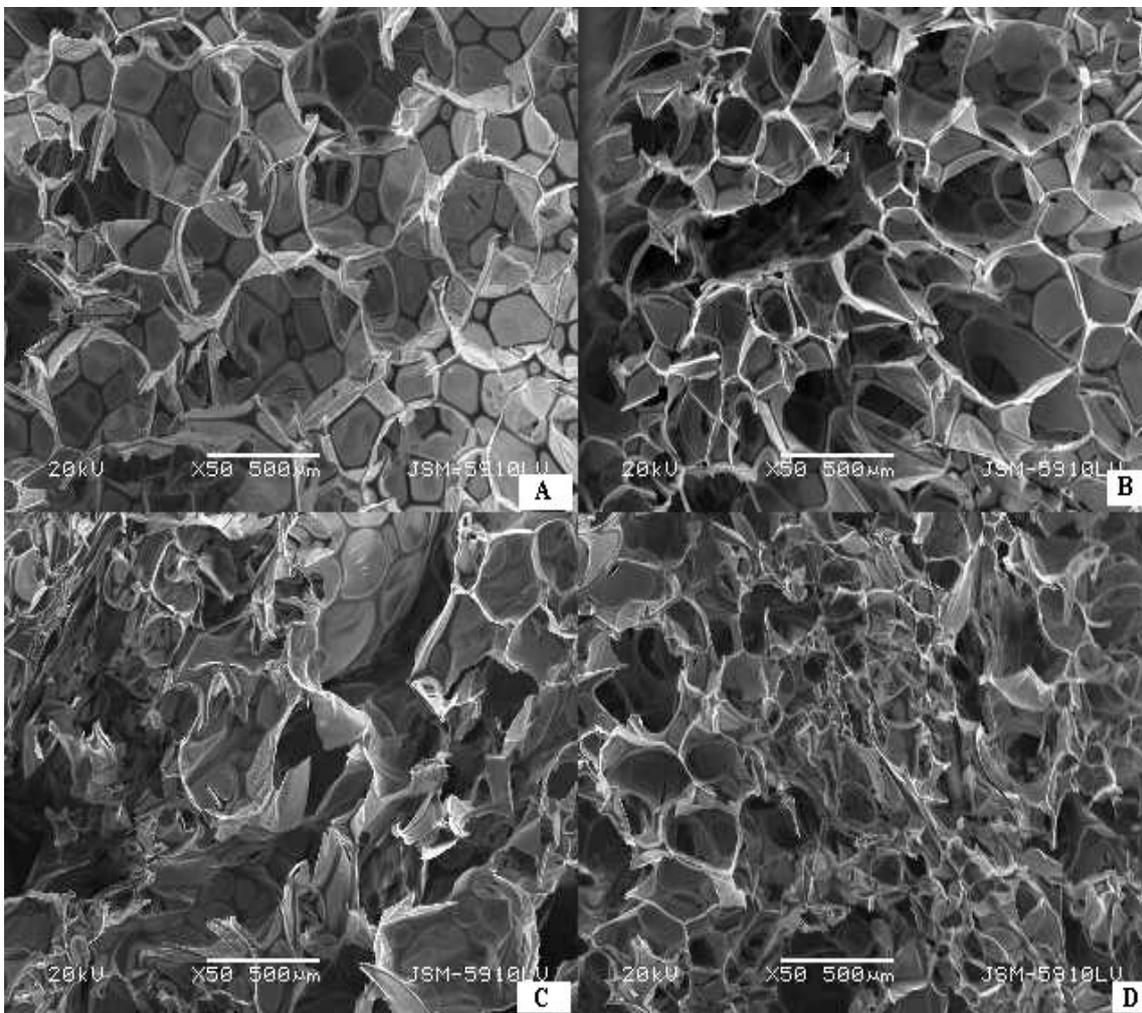
**Figure 7.** Cross-sectional SEM images of the PU foam with bamboo fiber additives (PUB). Magnification 50 x. A- standard PU foam, B- PU4B, C- PU8B, D- PU12B.
