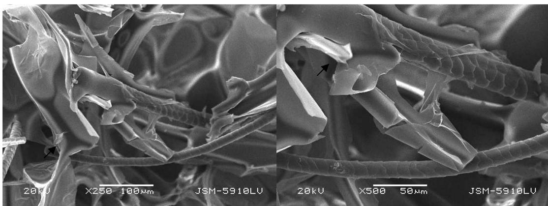
**Figure 10.** Cross-sectional SEM images of PU foam with wool fiber additives (PUW). Magnification 250 and 500 x.
