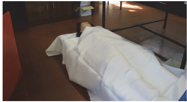
Figure 6. Thermal manikin measurements with the selected finished bed linens C and E
