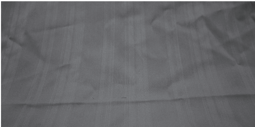
Figure 10. Fault on the fabric result from incorrect heat setting process parameters applied on the two for one twisted filament yarn (adapted from the reference of 30).
