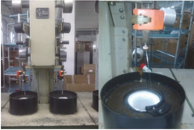
Figure 2. Socks knitting machines used.
