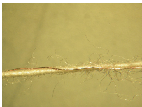
a. Copper-covered hybrid yarn
