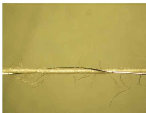
b. Stainless steel-covered hybrid yarn
