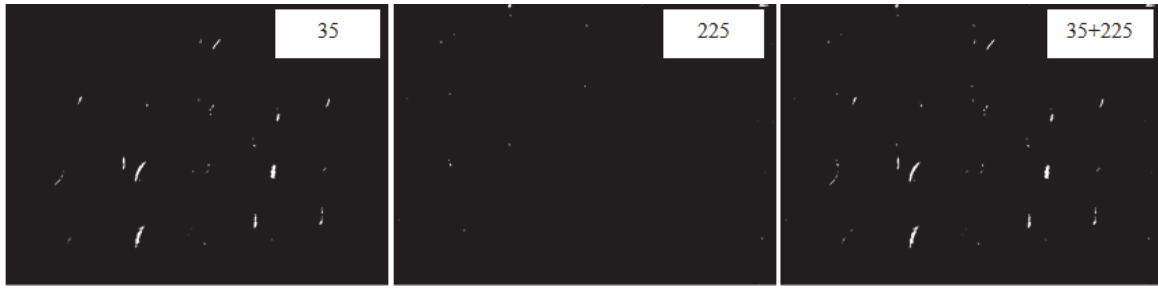
Figure 6. Results of image samples (30RC) of metals after thresholding at 35, 225, (35+225) pixel values.
