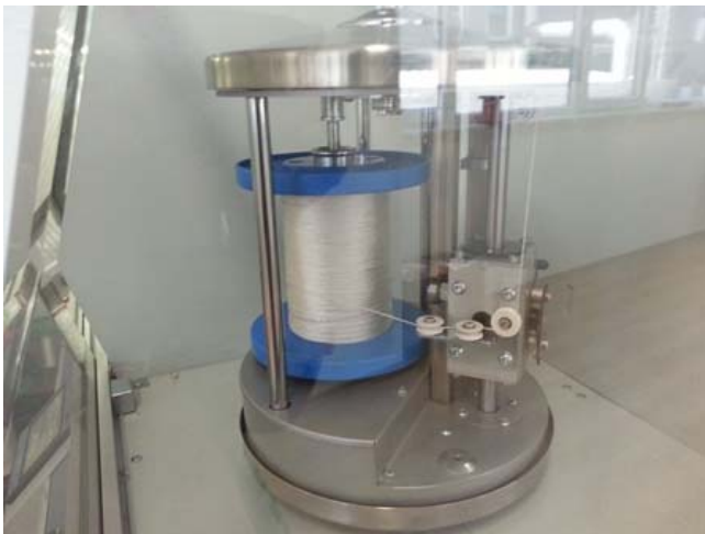
Figure 3. Production of composite yarn giving Z-twist
