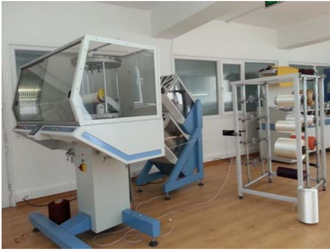
Figure 2. Plying process of sheath yarns in Agteks 2C-10" twisting machine
