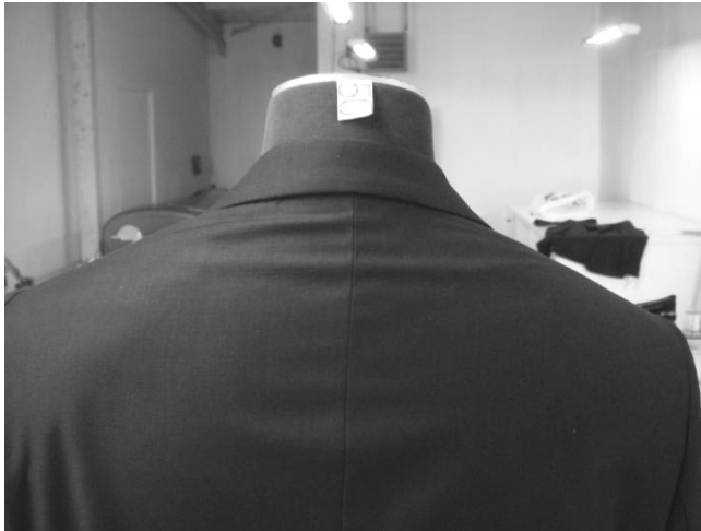
Figure 4.1. The Jacket Defect Related with Piling at the Nape Problem
