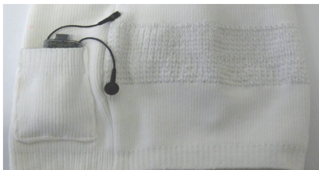
Figure 3. Detailed photograph of the shirt with battery and knitted heating elements.
