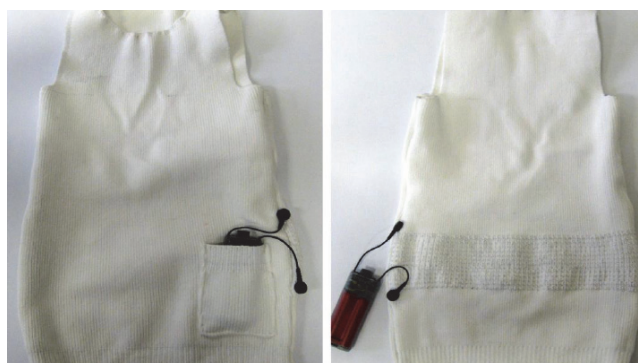
Figure 2. Photograph of a shirt with battery operated heating elements. Left: battery holder on the front side. Right: knitted heating element
