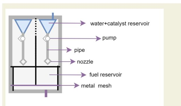
**Figure 2.** The design of the hydrogen generator system
