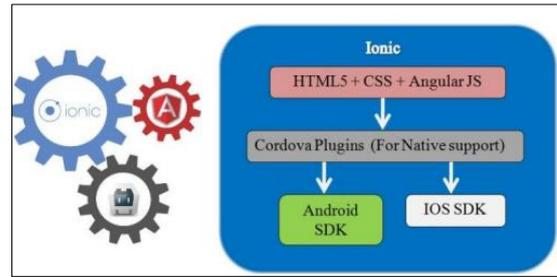
Figure 10. Ionic framework architecture [28]
