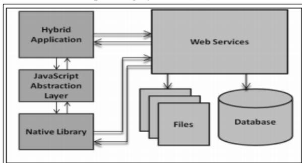
Figure 9. Hybrid mobile application process [27]
