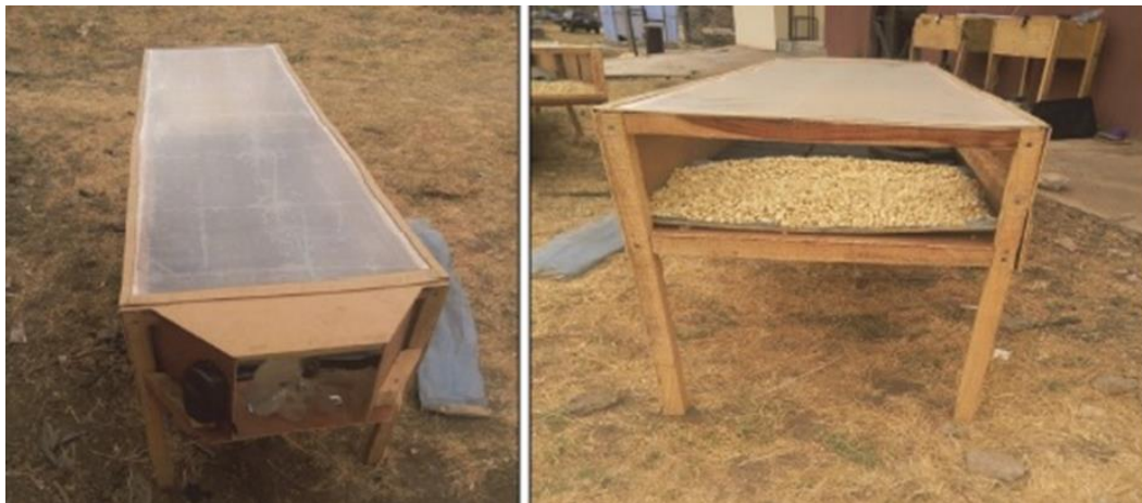
Figure 26. The direct-active desiccant crop dryer (Itodo et al., 2019).
