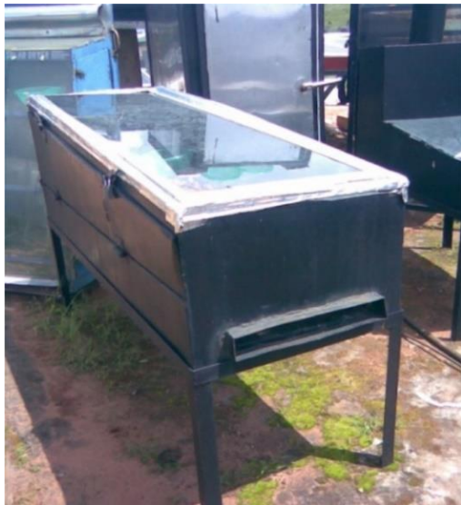
Figure 11. Latitudinal box solar dryer ( Eze and Ojike, 2012 ).
