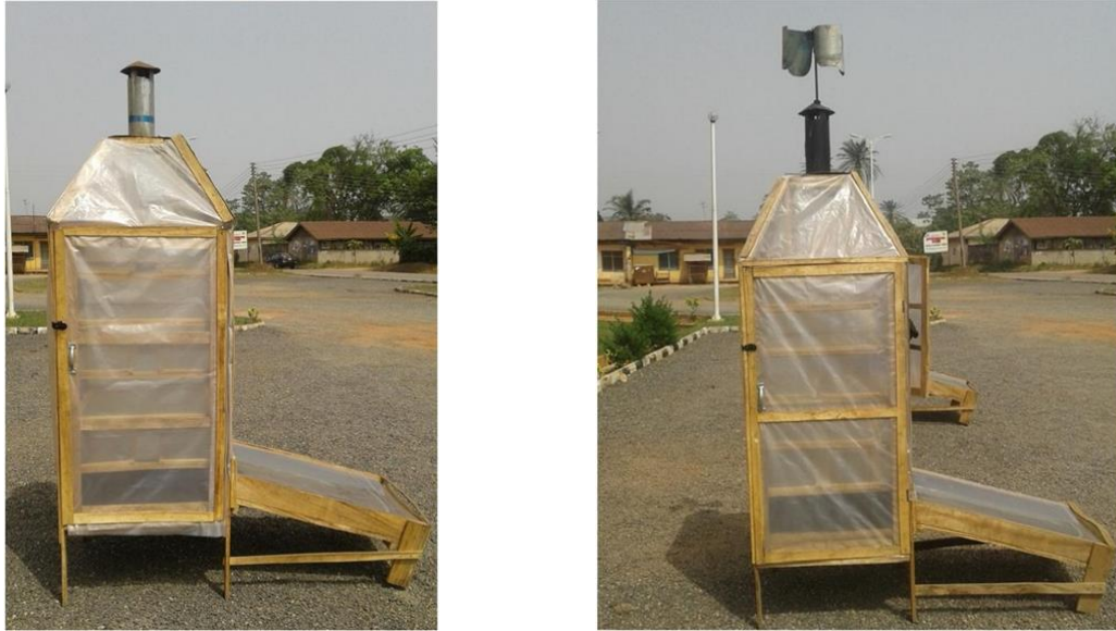
Figure 30. Developed prototype solar dryer without and with a wind generator ( Ndukwu et al., 2020a ).
