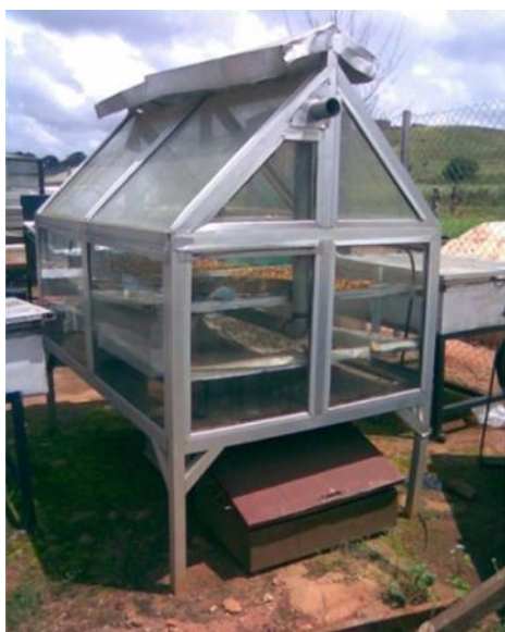
Figure 12. Greenhouse solar dryer ( Eze and Ojike, 2012 ).
