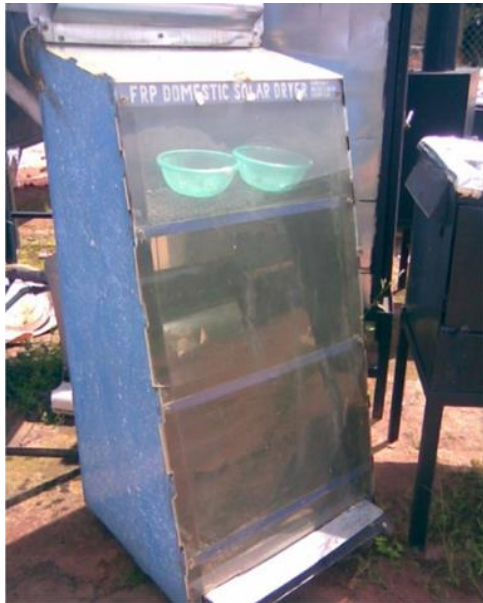
Figure 13. Sun manual tracking solar dryer ( Eze and Ojike, 2012 ).
