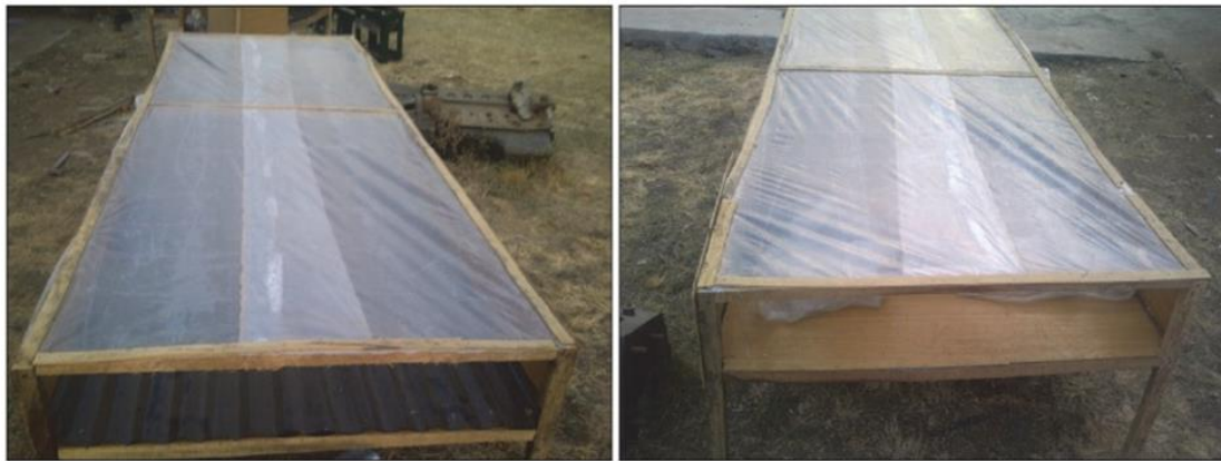
Figure 28. The direct-passive desiccant solar crop dryer (Itodo et al. , 2019).
