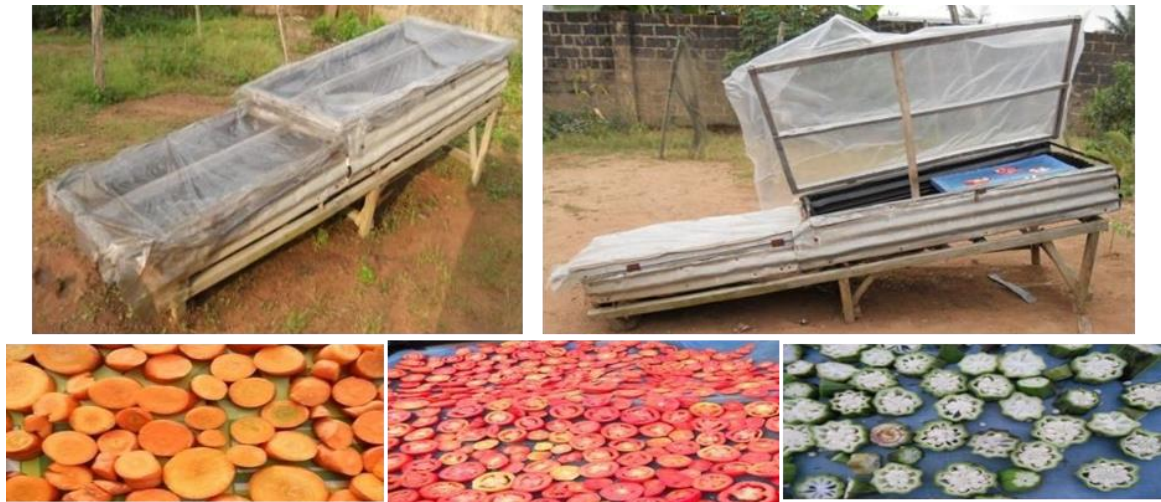
Figure 14. The direct mode natural convection solar dryer for carrot, tomato and okra (Eke, 2013).
