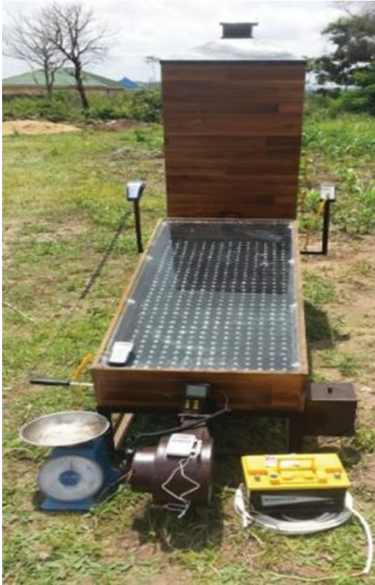
Figure 39. Complete assembly of the active transpired indirect solar cabinet dryer ( Kuhe et al. (2022) ).
