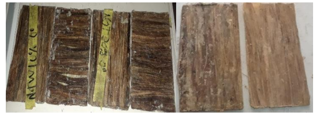
Figure 3. SSD fibre-epoxy composite produced at 0-degree and 90-degree orientation
