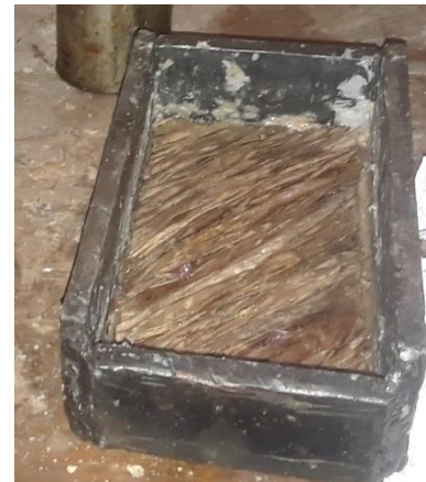
Figure 2. Fibre placed in the mould and a mixture of Epoxy/Hardener spread evenly on the fibres
