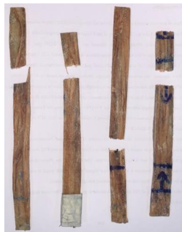
Figure 8. Fractures specimens of Hot Alkaline treated 5% SSD fibre at 0-degree Orientation
