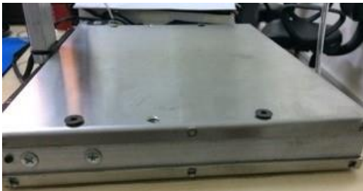
Fig. 2: Stainless chassis of the machine
