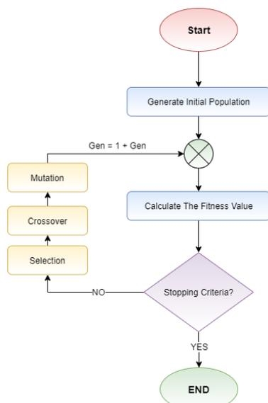
**Figure 2.** Flow chart of the genetic algorithms.
