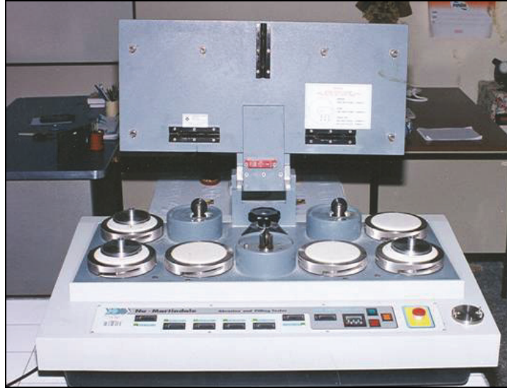
Figure 1. Martindale Pilling and Abrasion Tester (22)
