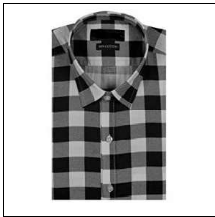
Figure 1. Check mismatch in shirt placket due to thermal shrinkage during fusing process
