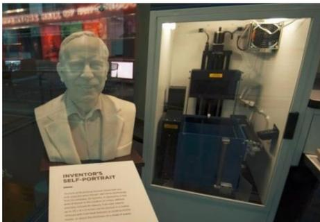
**Figure 1.** The first 3D printer invented by Charles (Chuck) Hull [4].
