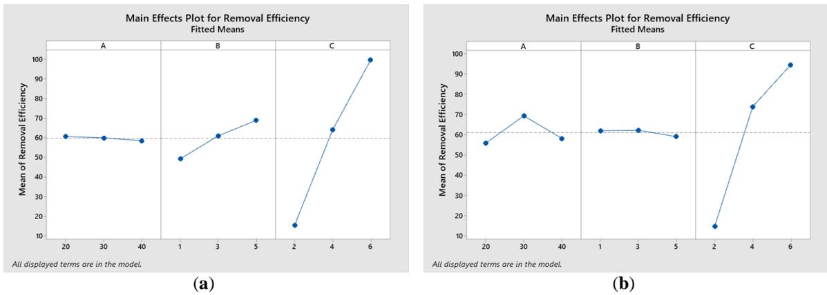
Figure 1. (a): Main effects Plot for Cr (III) on the Removal Efficiency. (b): Main Effects Plot for Pb (II) on the Removal Efficiency.
