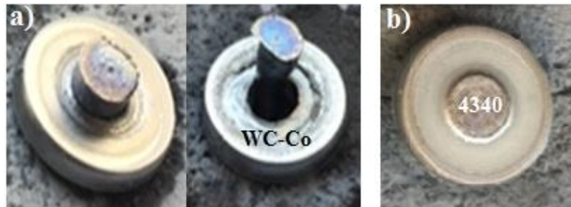
Figure 2. Sintered samples (a: 1350 °C, b: 1300 °C)
