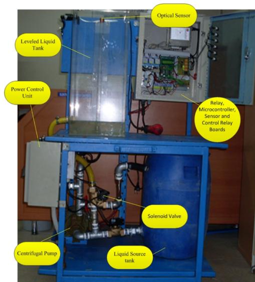
Figure 6. Mechatronic liquid level measurement system
