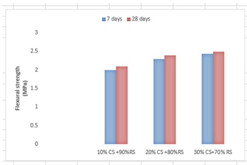
**Figure 2** Flexural strength of sand concrete
