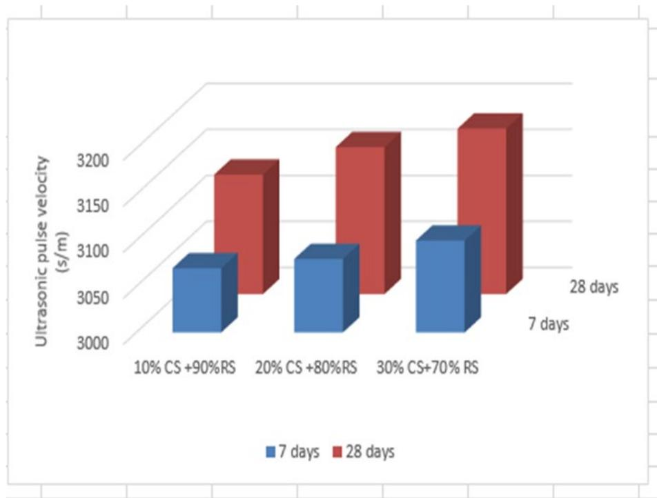
Figure 3 UPV of sand concrete
