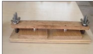
Figure 2. Bonding of test cylinders with the help of mold
