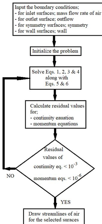
Figure 3. Flowchart for solution algorithm.
