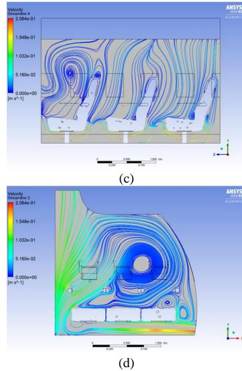
**Figure 8.** Air streamlines at different cross sections for DV case.
