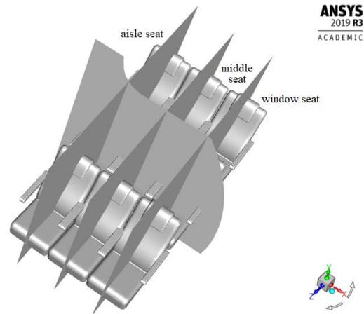
Figure 4. Cross sections from which air streamlines are visualized.
