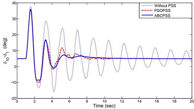
Fig. 6. The relative rotor angle of  $G_{10}$  under scenario 1.
