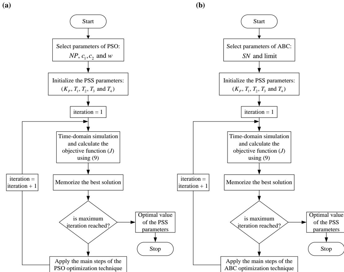
Fig. 2. (a) Flowchart of the PSO algorithm. (b) Flowchart of the ABC algorithm.
