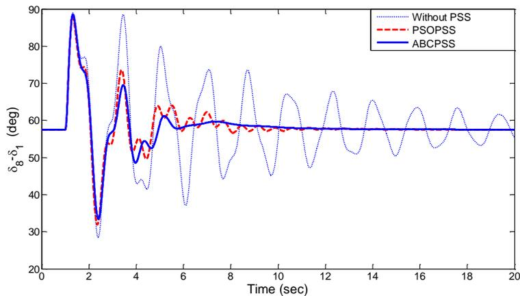
**Fig. 5.** The relative rotor angle of  $G_s$  under scenario 1.
