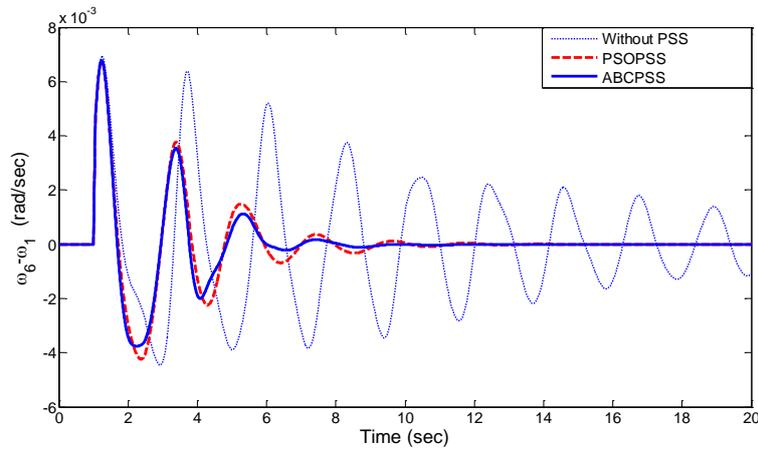
Fig. 11. The rotor speed deviation of  $G_6$  under scenario 2.
