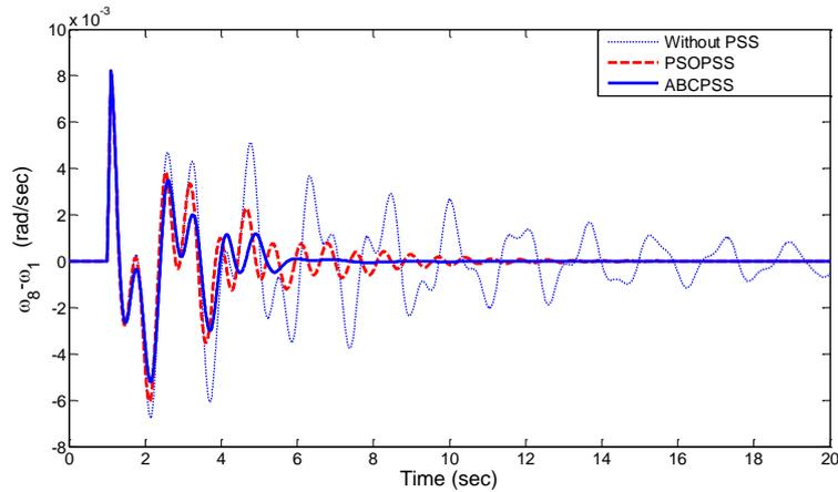
Fig. 7. The rotor speed deviation of  $G_8$  under scenario 1.
