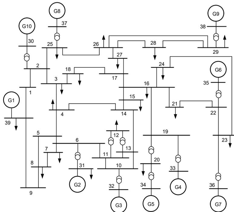
**Fig. 3.** New England 10-machine 39-bus power system.
