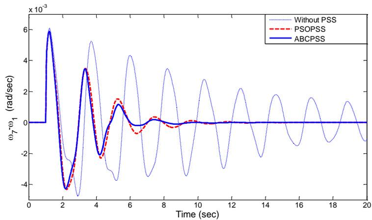
Fig. 12. The rotor speed deviation of  $G_7$  under scenario 2.
