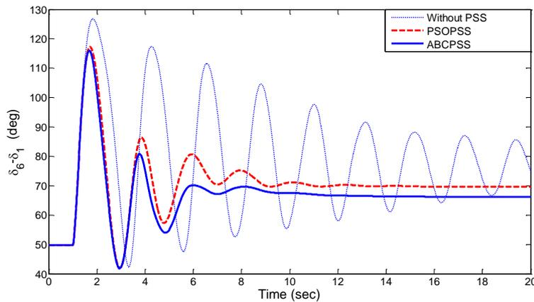
Fig. 9. The relative rotor angle of  $G_6$  under scenario 2.
