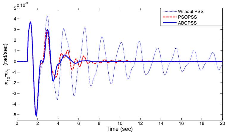
Fig. 8. The rotor speed deviation of  $G_{10}$  under scenario 1.
